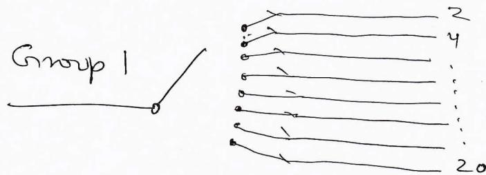
→ Interconnecting multiples of switches is called grading.
