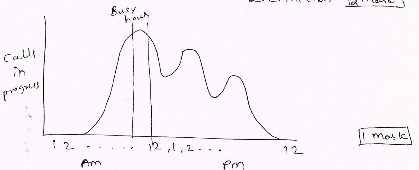
ii) Grade of Service - Probability of a call being blocked or queued for some period of time due to limited system resources during the busy hour of the day
