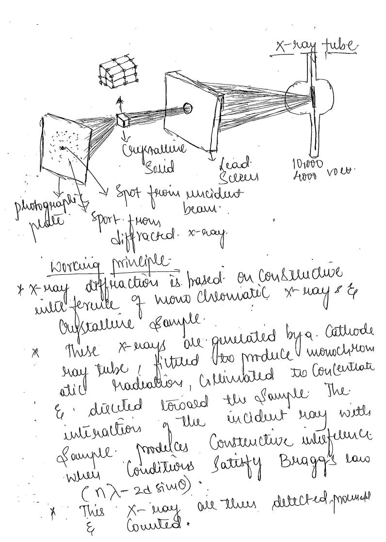
By & canning the Lample through a hange of 20 angles, all possible differentions directions of the lattice should be attained that the providence orientation of the possible material.
