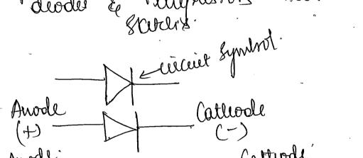
A diode is Fringly a PN junctions, but it's application are extensive in electronic circuit.
