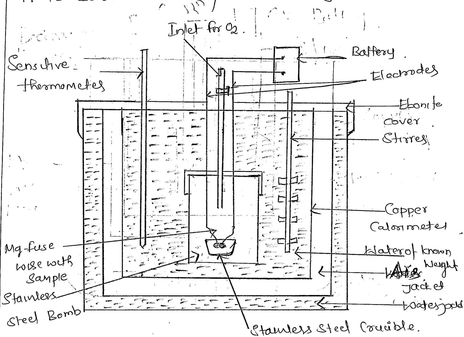
**Kloking:** The water is kept in constant agitation by the Mechanical stirrer. The initial temperature of the water is carefully measured. The fused magnesium wire is placed in the fuel. The Bomb is filled with oxygen. The fuel is ignited by connecting the two electrodes to a source of electric current. As the sample burns in the bomb
