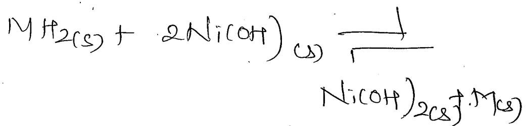
The cell has cell potential of 1.25 to 1.35V
