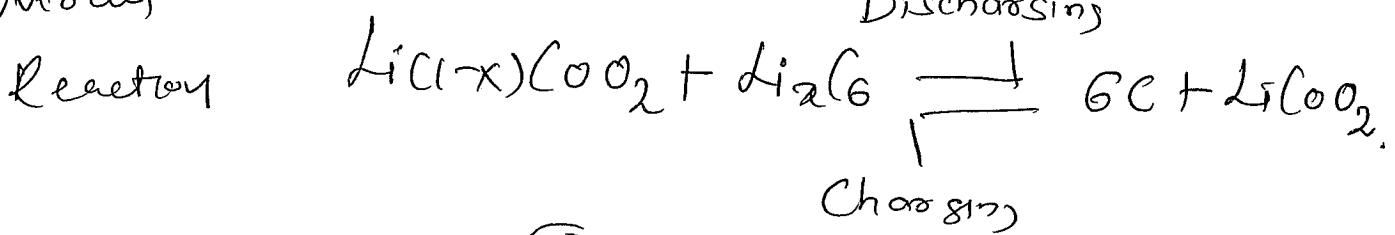
The unit cells are cylindrical and of jelly-roll design, usually of the same size as nicad (Ni-Cd) cells. The open circuit voltage is about 4.1V. Self discharge rate is about 10% per month.
