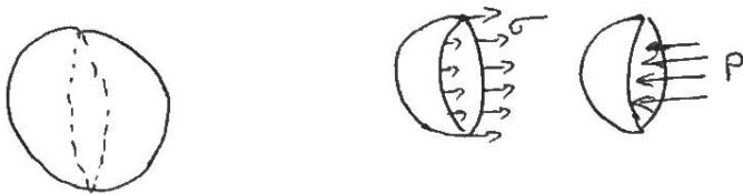
Consider a small spherical droplet of a liquid of radius 'r' on the entire surface of droplet the tensile force due to surface tension will be acting.
