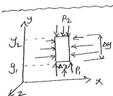
Consider a rectangular fluid element of height  $dy$ , length  $Ax$ , and unit depth ( $Az$ ) as shown in Fig.
