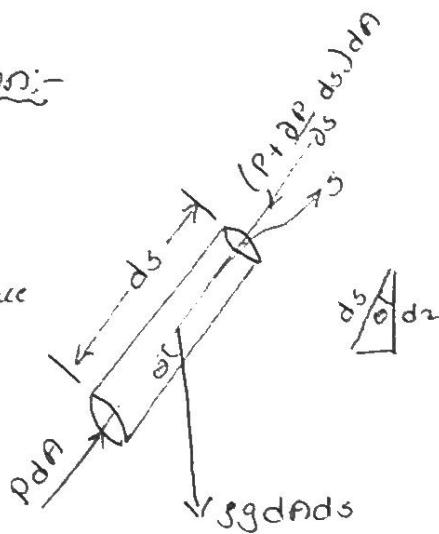
The forces acting on cylindrical element are
