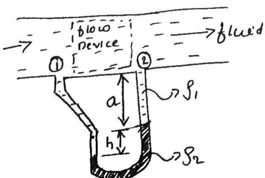
Manometers are particularly well suited to measure pressure drops across a horizontal flow
