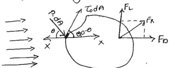
Consider an arbitrary shaped body placed in real fluid, which is flowing with a uniform velocity  $V$  in horizontal direction as show in fig
