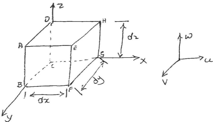
Consider a fluid element of length  $dx$ ,  $dy$ ,  $dz$  in directions of  $x$ ,  $y$ ,  $z$  respectively. Let  $u$ ,  $v$ ,  $w$  are velocity at inlet in  $x$ ,  $y$ ,  $z$  directions.
