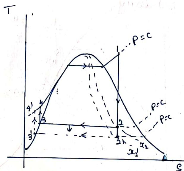
→ If condenser pressure decreased, the turbine work ( $h_1 - h_2$ ) increases to ( $h_1 - h_2'$ ).
