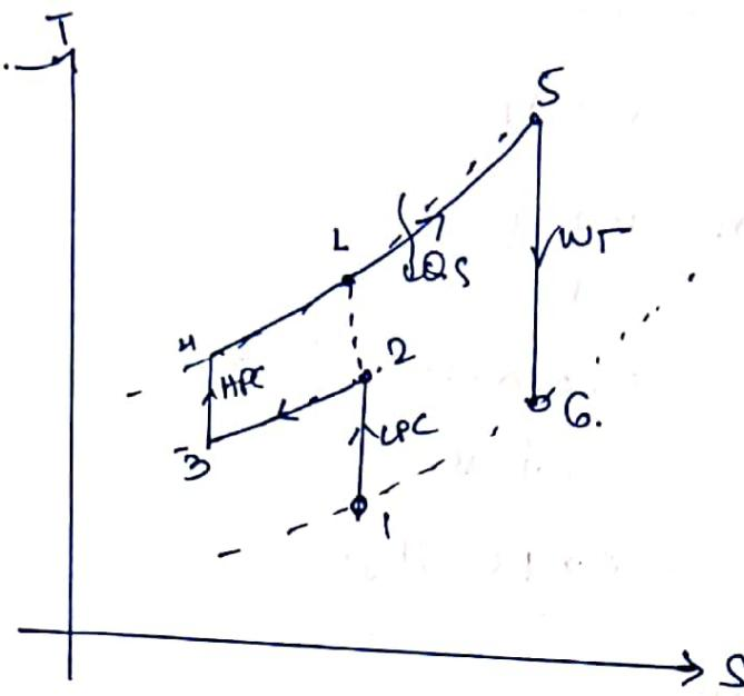
The compressor in a gas turbine cycle utilizes the major percentage of power developed by the gas turbine. The work required by the compressor can be reduced by compressing the air in two stages & by incorporating intercooler between the two as shown.
