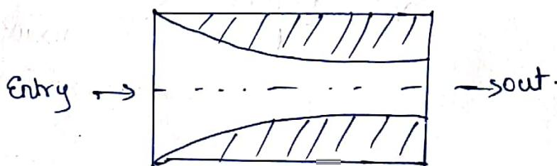
In this nozzle, the cross sectional area decreases continuously from its entrance to exit. It is used in a case where the back pressure is less than the critical pressure ratio.
