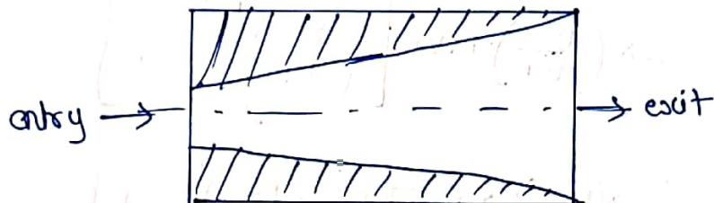
The cross sectional area of the divergent nozzle increases continuously from its entrance to exit.
