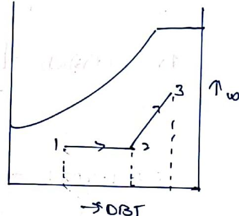
In the heating / humidifying process, the air first passes through a heat exchanger & then through the humidifier where steam is sprayed into the air stream.
