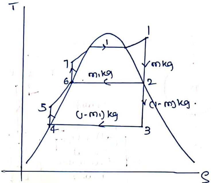
The steam leaving the boiler enters into the turbine at state 1. The part of the steam say  $m \text{ kg}$ , is expanded to state 2 only of this steam enters the feed water heater. the remaining  $(1-m) \text{ kg}$  of steam after the turbine enters into the condenser & is condensed. The condensate is then pumped to the feed water heater. Here it mixes with the steam extracted from the turbine. Thus feed water gets heated from 5 to 6 & is then pumped by another pump to the boiler pressure.
