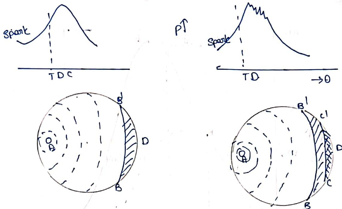
A normal flame front travels across the combustion chamber from A towards D. in normal combustion. If, however, the flame front is able to proceed only as far as, say C'C, during the ignition delay period, then the remaining portion of the unburned charge C'D will auto-ignite & cause extreme pressure fluctuations. This causes severe pressure waves which strike the cylinder wall & set it vibrating, giving rise to a characteristic high pitched metallic sound. called detonation.
