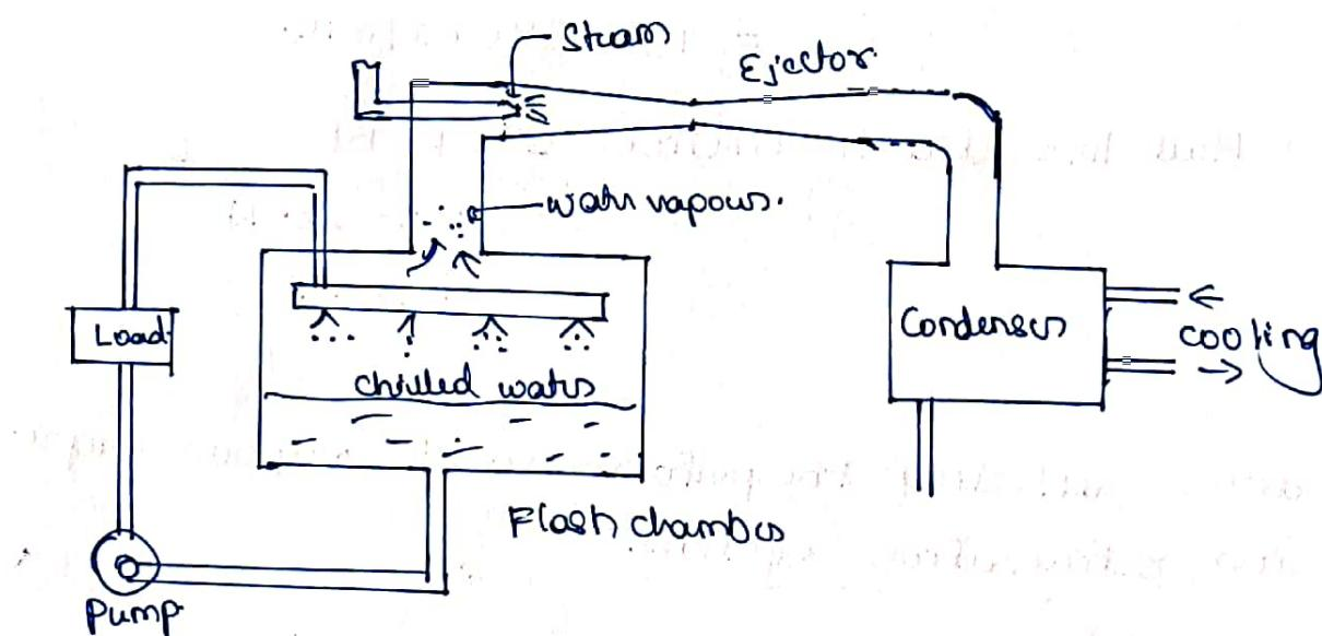
→ Steam from the boiler also called motive steam expands through the nozzle. The high velocity vapour imparts the momentum to the vapour in the flash chamber & thus the vapour moves along with the motive steam through the ejector.
