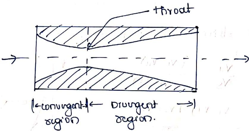
The cross sectional area of nozzle first tapers to a smaller section; being throat, & then it diverges to a large diameter. The nozzle which converges to throat & diverges afterwards is known as convergent-divergent nozzle.
