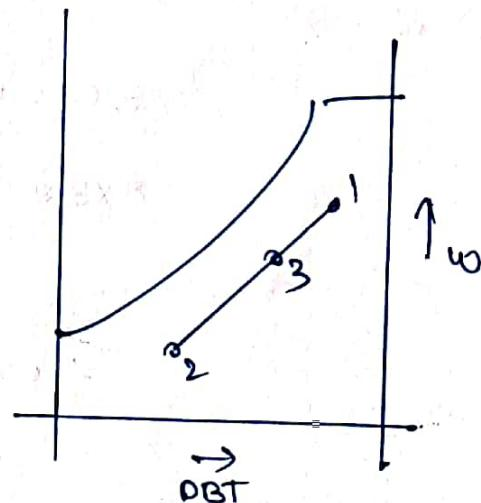
Two air streams of different Psychrometric properties are mixed together. Then the Psychrometric properties of the mixture can be calculated by balancing the enthalpies of mass of water vapour.
