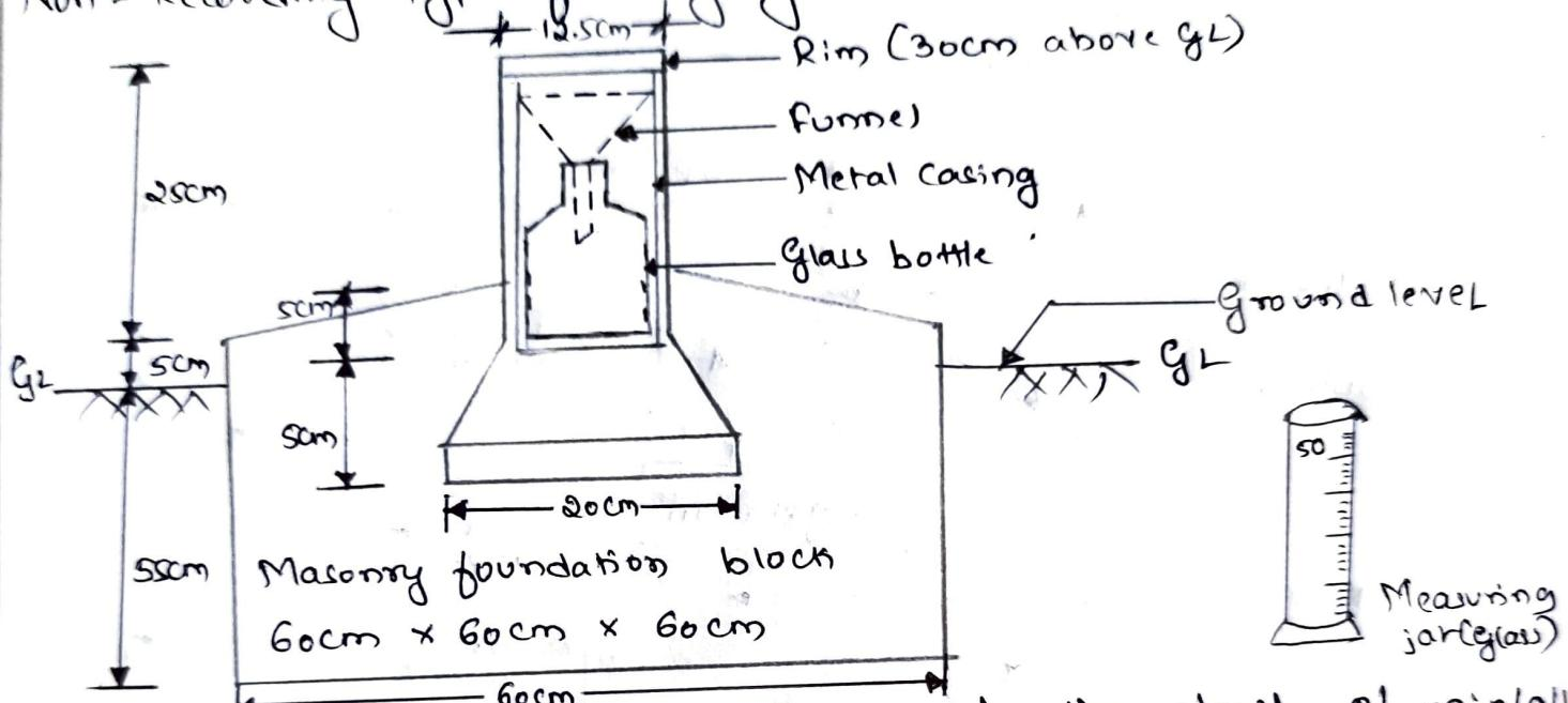
These rain gauges which do not record the depth of rainfall but only collect rainfall. Symons rain gauge is the used non recording type of rain gauge. It gives the total rainfall that has occurred at a particular period. It essentially consists of a circular collecting area 107mm in diameter connected to a funnel. The funnel discharges the rainfall into a receiving vessel. The funnel and the receiving vessel are housed in a metallic container. The components of this rain gauge are on the figure.
