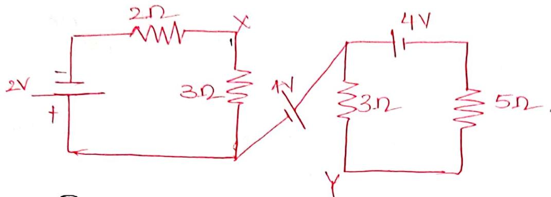
$$I_1 = \frac{2}{2+3} = 0.4 \text{ A} \quad \& \quad I_2 = \frac{4}{3+5} = 0.5 \text{ A}$$
