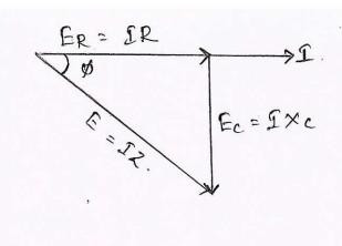
From the vector d'agram, we observe that the arrent leads the voltage by an angle of.
