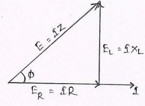
The vector diagram consult of three voltages, ER = IR which in inphase with current, EL = IXL which leads current by 90°. The vector sum of these two voltages in the applied voltage E = IZ, where Z is impedance of the circuit.
