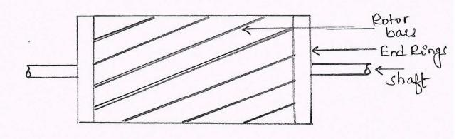
It consist of cylindrical laminaled core with parallel slots for carrying heavy base of copper or aluminium rotor conductors. The slots are slightly skewed, which helps in two ways. is it reduces noise due to magnetic hum of makes the rotor to run quietly. it reduces the locking tendency between rotor of stator.
