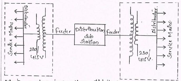
Most modern low voltage distribution systems are operated at Ac rated voltage of 230/4150 at 50 the in lindia.
