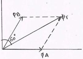
It in observed that resultant flux has notaled by 60° in the clockwise direction of its magnitude is
