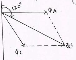
The runtant flux has notated by another 60° ie through 120° from îts original position of its roagnitude is 150m
