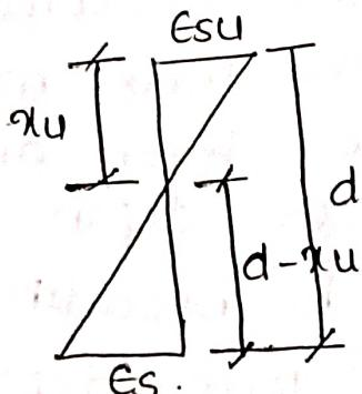
To avoid compression failure, IS 456 recommends strain corresponding to 0.0035
