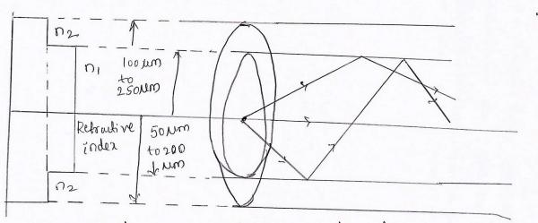
I Step index fibres which have core diamiters in the range of 2µm to cours are known as single mode Stepindex fibres. I These fibres essentially transmit only the axial mode due to very small core diameter I The Thickness of the core is typically 2surp to 30µm These fibres are used for long distance compoundation as intermodal dispersion is eliminated.
