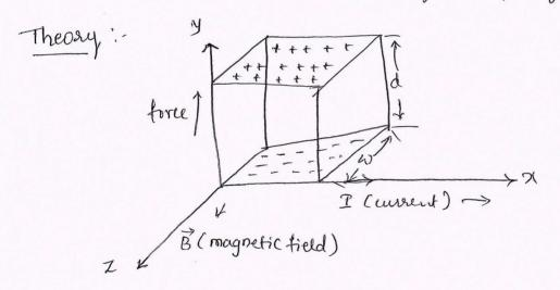
consider a rectangular slab of a Seroi conductor material in which a censent I is flowing in the positive 2-direction. Let the servi conducting material be of n-type, which
