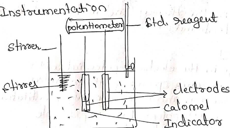
Potentiometer consists of one indicator electrode, a reference electrode & a potentiometer to measure the cell potential
