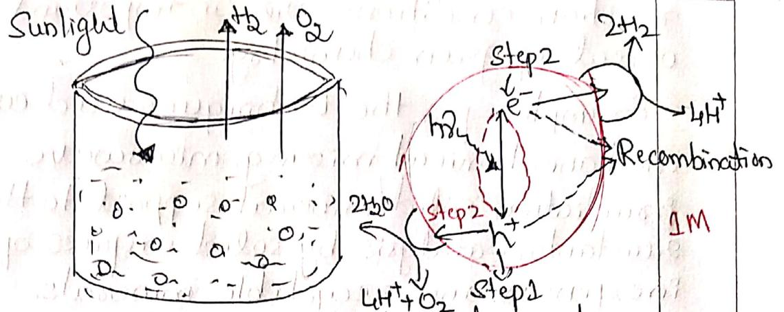
→ Splitting of water to get hydrogen by using a photocatalyst & using solar energy is called photocatalytic water splitting.
