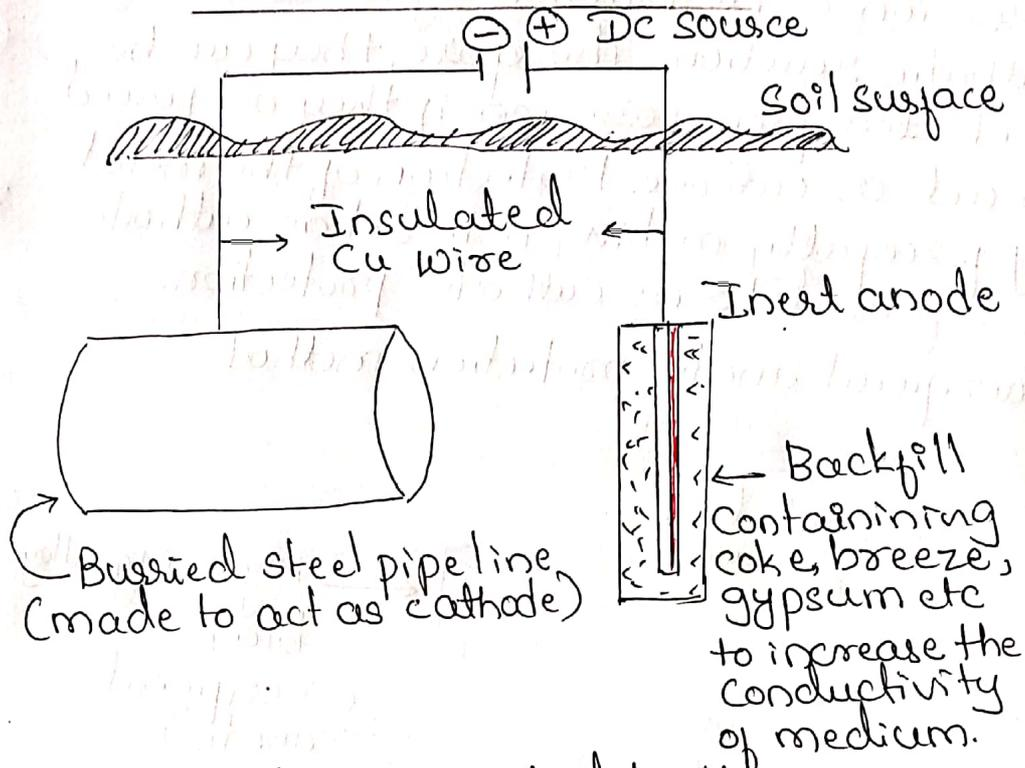
→ Object metal is connected to the -ve terminal of an external DC source with higher potential and is made as cathode.
