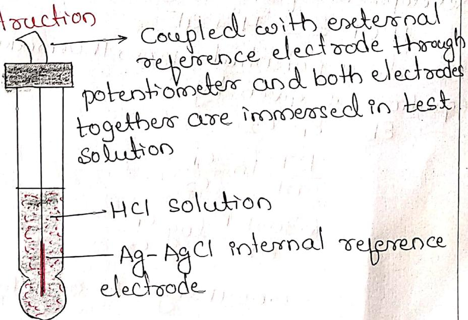
A glass membrane electrode consists of a specially made glass membrane extending out as a bulb at the end of a plane glass tube containing Ag-AgCl electrode immersed in a solution of HCl. 1M
