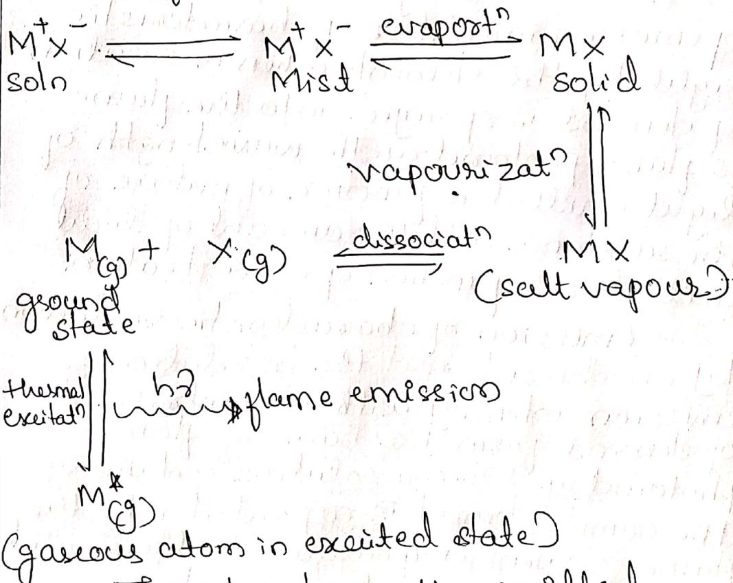
The intensity of the emitted radiation, measured as detector response is related to the analyte concentration by an expression:
