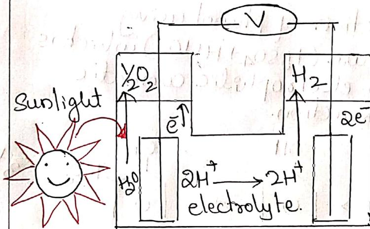
The light energy excites an electron ( $e^-$ ) in the semi conducting material (electrode). Thus produced hole ( $h^+$ ) will react with the neighbouring  $H_2O$  molecule.
