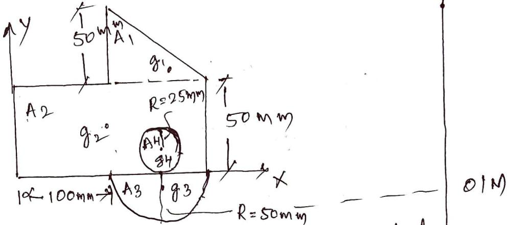
Let  $A_1, A_2, A_3$  &  $A_4$  be the segmental areas of given composite section. Let  $g_1, g_2, g_3$  &  $g_4$  be the positions of centroids of  $A_1, A_2, A_3$  &  $A_4$  respectively.
