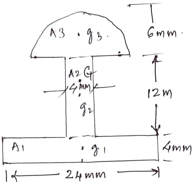
Let  $A_1, A_2 \text{ & } A_3$  be the segmental areas &  $g_1, g_2 \text{ & } g_3$  be the positions of centroids of  $A_1, A_2 \text{ & } A_3$  as shown in figure.
