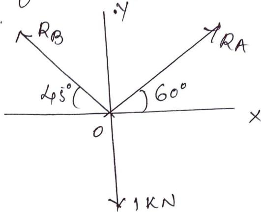
Let  $R_A$  &  $R_B$  be the reactions at contact points A & B respectively.
