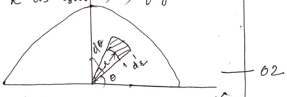
Due to symmetry Centroid must lie on the y-axis. Let its distance from diametral axis by  $\bar{y}$ . To find  $\bar{y}$ , consider an element at a dist.  $\theta$  from the centre O of the semicircle, radial width being  $d\theta$  and bound by radii at  $\theta$  &  $\theta + d\theta$ .
