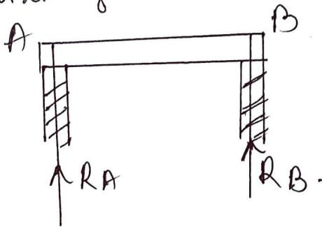
Roller Support: It is a support in which the ends are free to roll on support; there is no resisting moment developed. The reaction is normal to the axis of the structural member.
