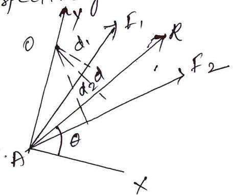
Let O be the moment centre, join OA & consider it as Y-axis and to it draw X-axis as shown. Let  $\theta$  be the inclination of R with X-axis.
