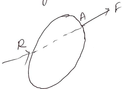
As per principle of transmissibility the state of rest is unaltered if  $F$  is replaced by  $R$  but  $R$  should in the same direction & it should be along the line of action of  $F$  as shown in fig.
