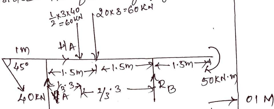
Let  $V_A$  &  $H_A$  be the vertical & horizontal components of reaction in any direction due to hinged support at point A &  $R_B$  be the normal reaction due to roller support at pt B.
