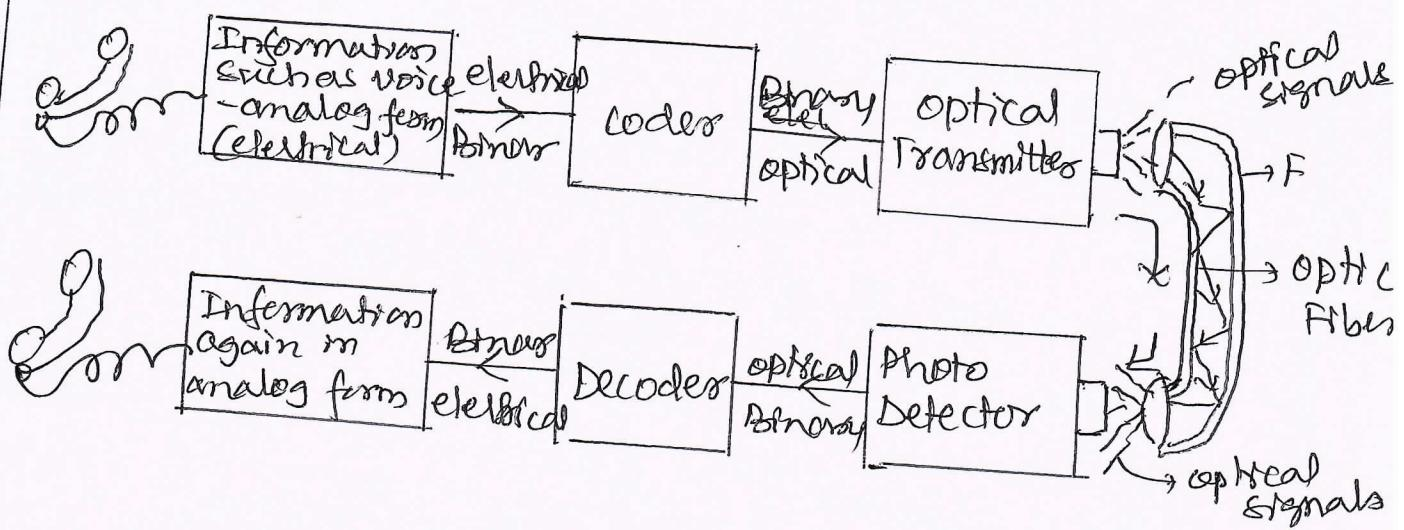
In an optical fiber communication system, the input signals (audio, video or other digital data) are used to modulate light from a source like a LED or a semiconductor LASER & is transmitted through optical fiber. At the receiving end the signal is demodulated to reproduce the input signal. If data transfer takes place between only two devices then, it is called point to point communication.
