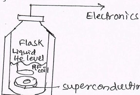
superconducting loop with a weak link
