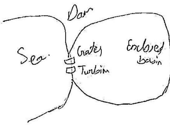
Gate is large enough to admit the water during tide so that the loss of head is small is provided in the dam.
