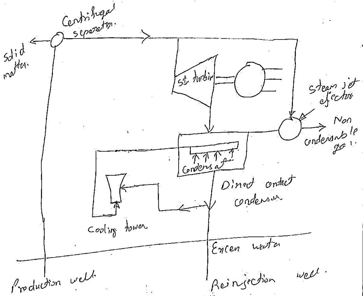
In dry steam plant, steam produced directly from the geothermal reservoir runs the turbines that power the generator.
