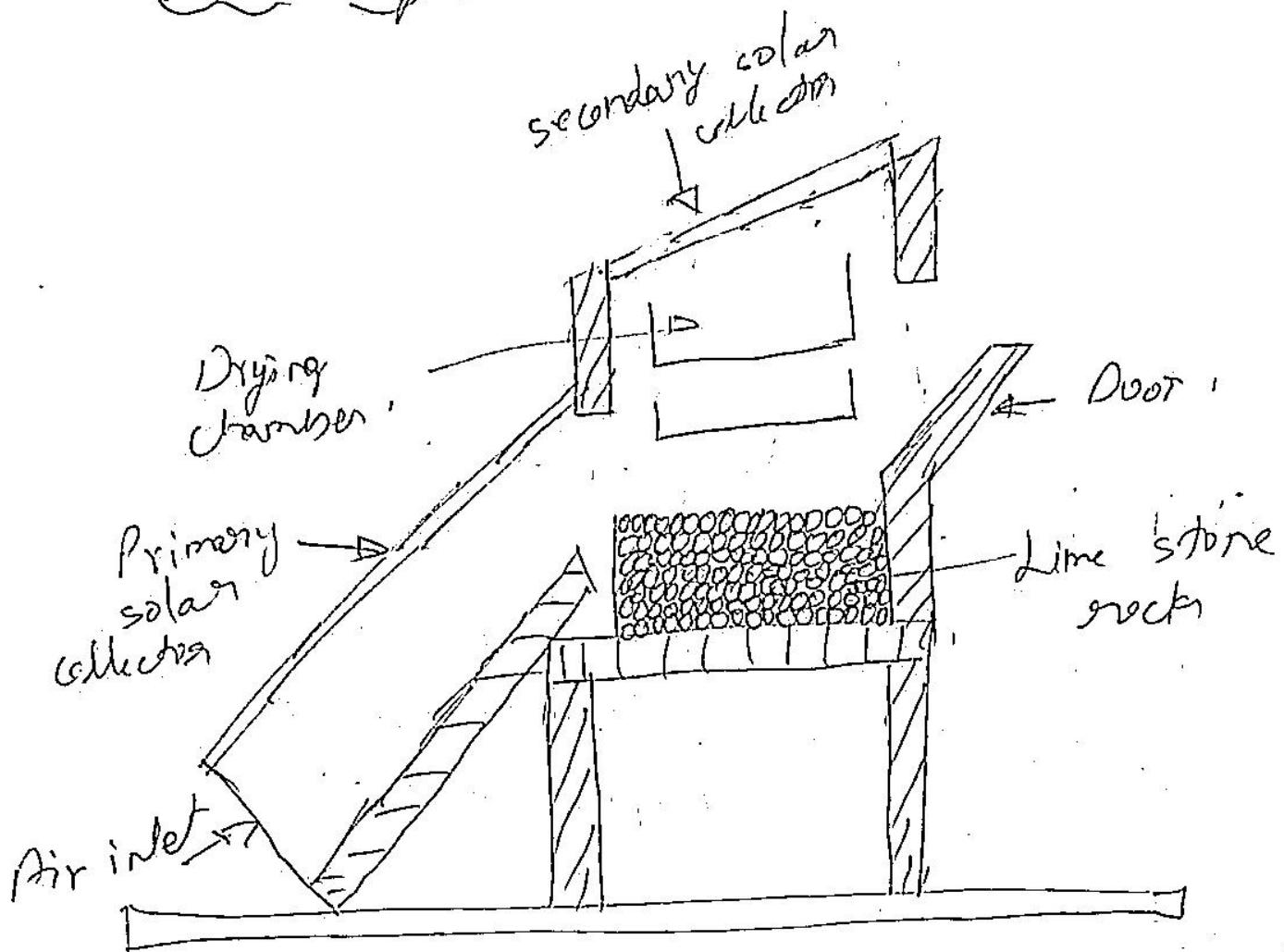
In a rock bed solar dryer, air drawn by natural convection through an air inlet (A), circulates the heat collected by the primary solar energy. The heat collected by the primary solar energy is transferred throughout the drying chamber, which is packed with limestone rocks of relatively uniform diameter. The heat would then stratify a given diameter. The samples positioned above the rock bed can continue drying during the night.
