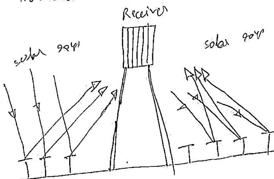
Heliostat is a mirror based system that is used continuously to reflect sunlight onto a central receiver. The collected solar is then converted into electrical power.
