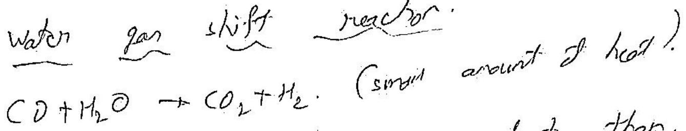
The process is typically much faster than the steam reforming & requires a small reactor vessel.
