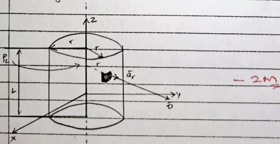
Consider differential surface area  $ds$  as shown which is at the radial distance  $r$  from the line charge.
