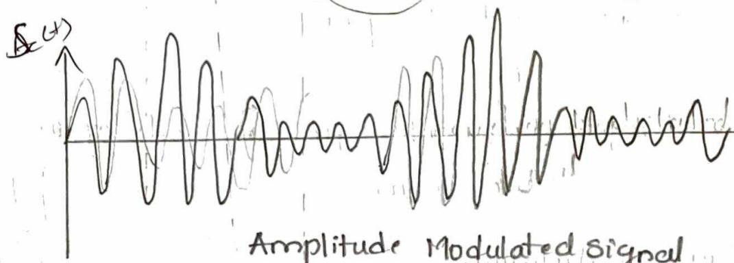
Amplitude Modulated Signal
