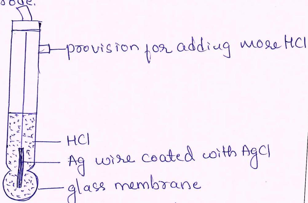
→ A glass membrane electrode or pH sensor consists of a specially made glass membrane extending out as a bulb at the end of a plane glass tube containing Ag-AgCl electrode immersed in a solution of HCl.
