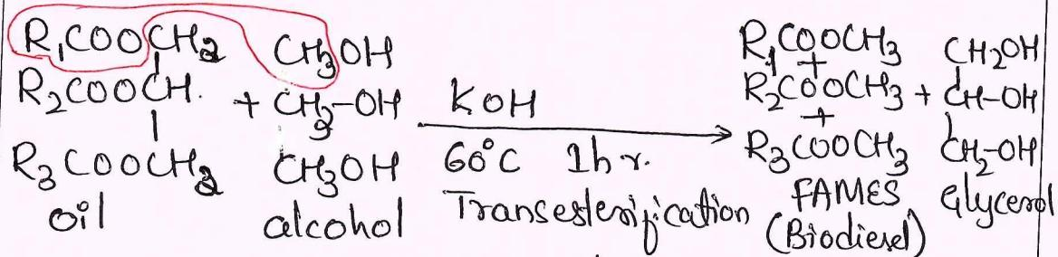
Glycerol is separated from the bottom of the reactor and organic layer containing mixture of FAMEs is washed with  $\text{H}_2\text{O}$ , dried over anhydrous  $\text{Na}_2\text{SO}_4$  and used as biodiesel.
