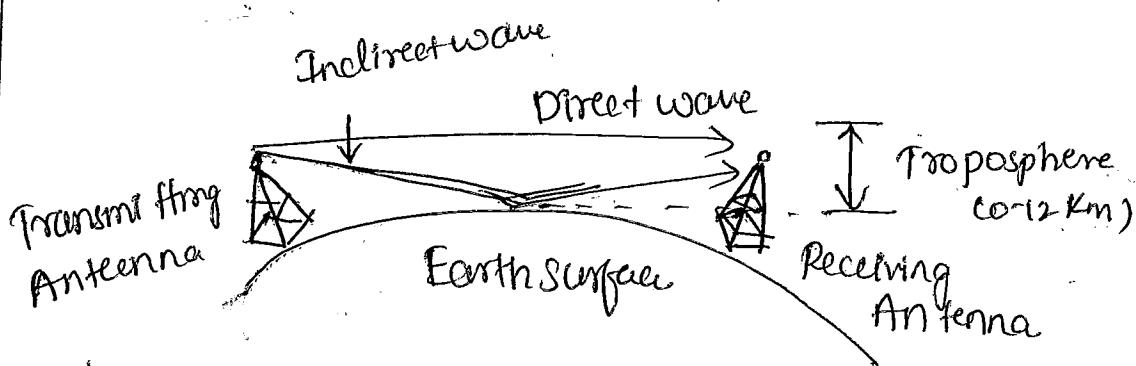
The space wave is made up of two components:
