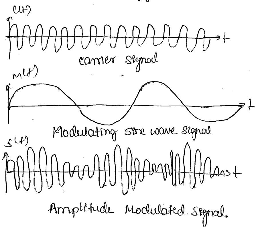
The first figure is the carrier wave, which is a high frequency signal and contains no information. Denoted as
