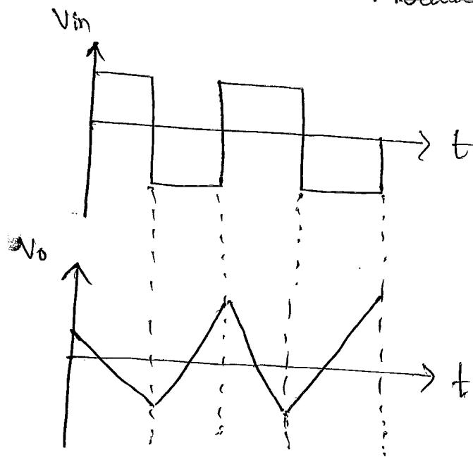
The circuit provides opposite function to that of difference here o/p is equivalent to area under the graph (input function).
