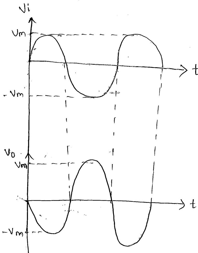
Here i/p signal is applied to I i/p terminal via  $R_1$ , Non I be ground via  $R_2$ .  $R_f$  is applied to connected b/w output & input side. Since i/p signal to inverting terminal is called Inverting Amplifier
