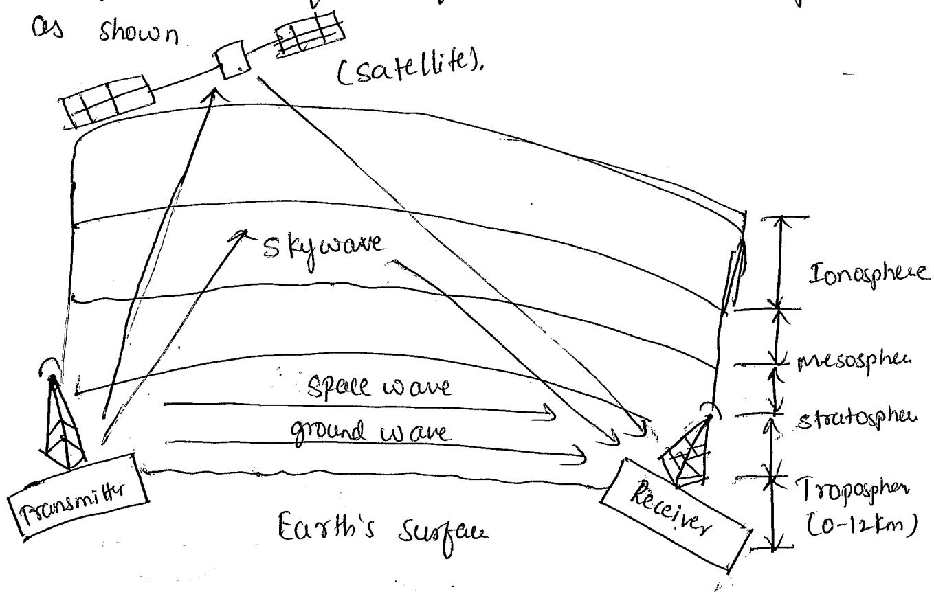
Sky wave is responsible for short wave transmission around the globe via successive reflections at the ionosphere and the earth's surface.
