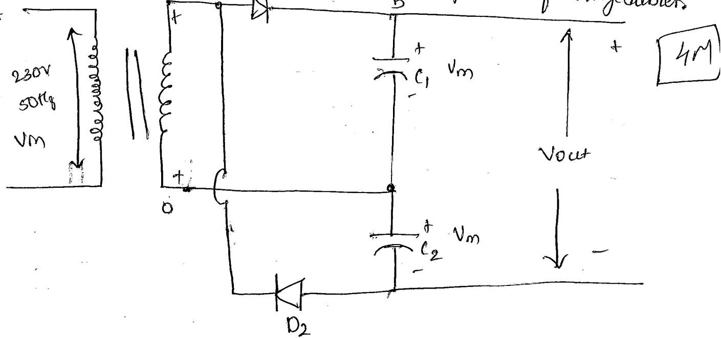
During the + half cycle diode D<sub>1</sub> is forward biased and D<sub>2</sub> is reversed biased
