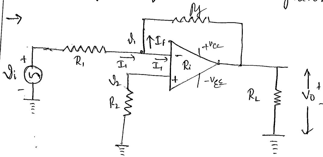
Applying KCL at  $V_1$
