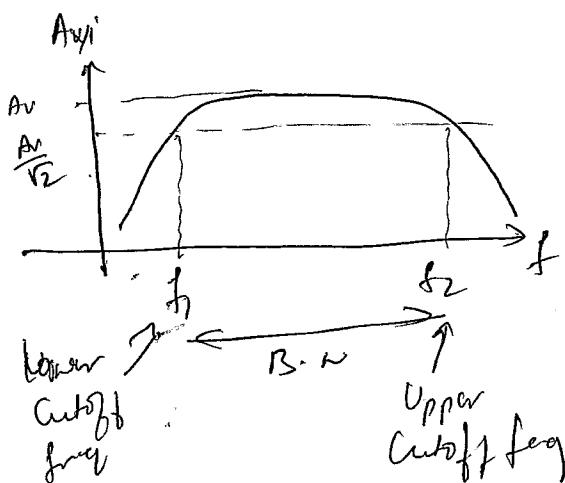
frequency Response indicates range of frequency over which gain drops 70.7% of its mid band value
