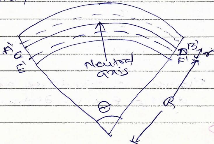
Consider a long uniform beam MN whose one end is free at N. The beam can be thought of as made up of a number of parallel layers like AB, CD, EF ... etc.
