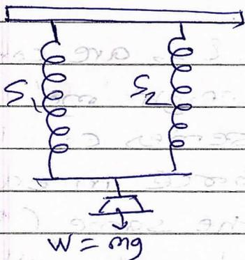
Suppose two springs  $S_1$  &  $S_2$  are connected in parallel combination. When springs are in parallel, each spring will undergo same amount of extension 'y'. However, the restoring force developed in two springs will be different as they have different spring constants
