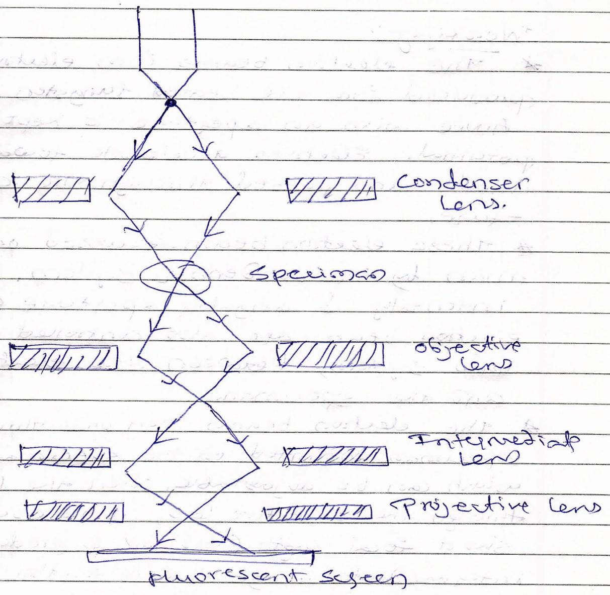
Construction:- TEM is an electron microscope that has four main parts
