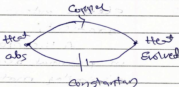
If a current flows through a circuit containing junction of two dissimilar metals, it leads to an absorption or liberation of heat at the junction.
