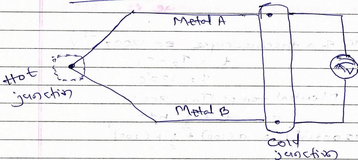
Thermocouple is constructed by joining wires made from dissimilar metals to form a junction. Voltage is produced when the temperature of the junction changes. Sensitive voltmeter is used to measure thermo EMF.
