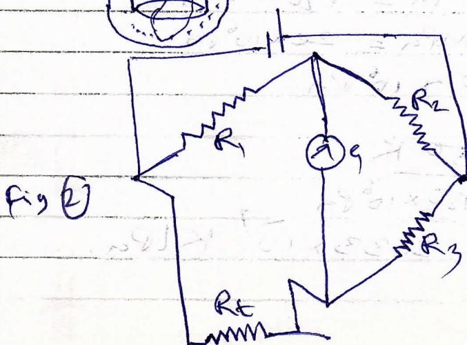
The PRT consists of pure platinum wire wound on hollow pipe made up of insulating mica or ceramic, which is placed in porcelain sheath. Free ends of the platinum wire are attached to long leads of low resistance copper wires. To measure change in resistance, Wheatstone bridge is used. Two long extension leads form one arm of wheatstone bridge.
