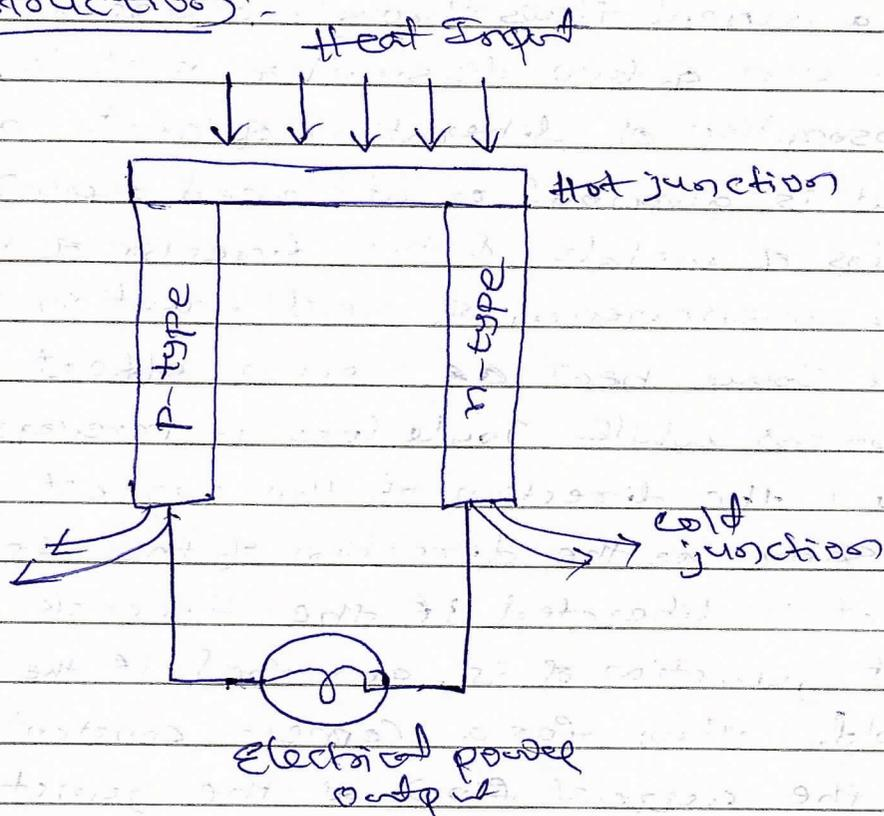
The simplest TEG consists of a thermocouple comprising a p-type & n-type thermo-element connected electrically in series and thermally in parallel. The p-type & n-type semiconductors are interconnected through a metal. Load is connected to free end of p & n-type semiconductors.
