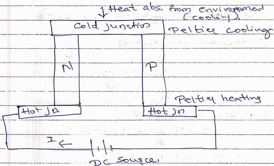
Thermoelectric cooling is a way to remove thermal energy from a medium, device or component by applying a voltage of constant polarity to a junction between two dissimilar semiconductors. Thermoelectric cooling uses the Peltier effect to create heat flux between the junction of two different type of materials. The device has 2 sides & when a DC electric current flows through the device, it brings heat from one side to the other, so that one side gets cooler while the other gets hotter.
