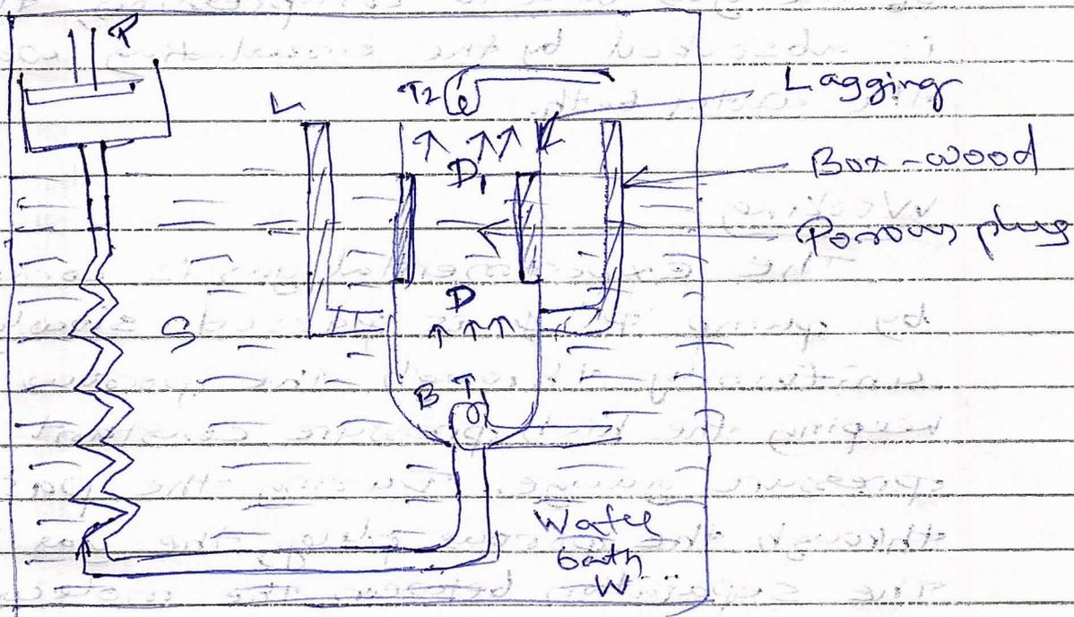
Construction: Joule in collaboration with Thomson devised a very sensitive technique known as porous plug experiment. The experiment is set up to study Joule-Thomson effect.
