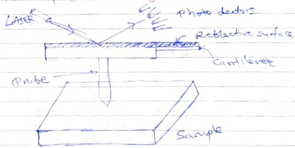
Principle:- Atomic Force Microscope (AFM) produces image by physically pushing a cantilever probe against the sample. The probe movement is analysed & converted into 3D image of the sample surface.
