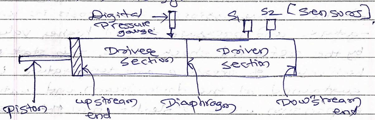
Construction:- Reddy's tube consists of a cylinder made of stainless steel tube of about 30mm in diameter & of length nearly 1m. It is divided into two sections each of length 50cm. The two are separated by 0.1mm aluminium or paper diaphragm. The tube has a piston fitted at far end of the driver section whereas the far end of the driven section is closed.
