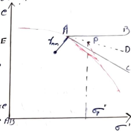
**UNDER CONSOLIDATED SOIL:** A soil which is not fully consolidated under the existing over burden pressure is called an under-consolidated soil.
