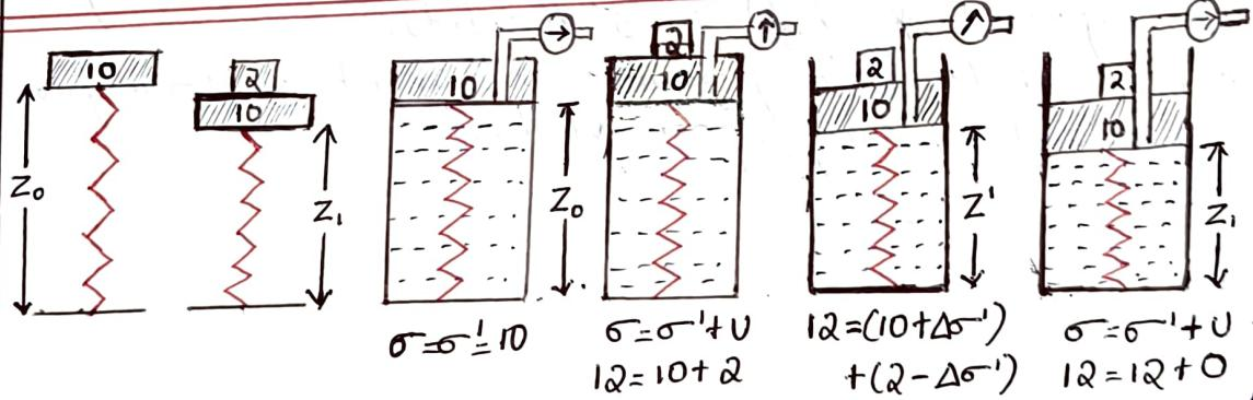
Consider a spring with a piston on its top. Let the length of the spring be  $Z_0$  under a pressure of 10 units. If extra 2 units is added the spring will be compressed immediately to a length  $Z_1$ .
