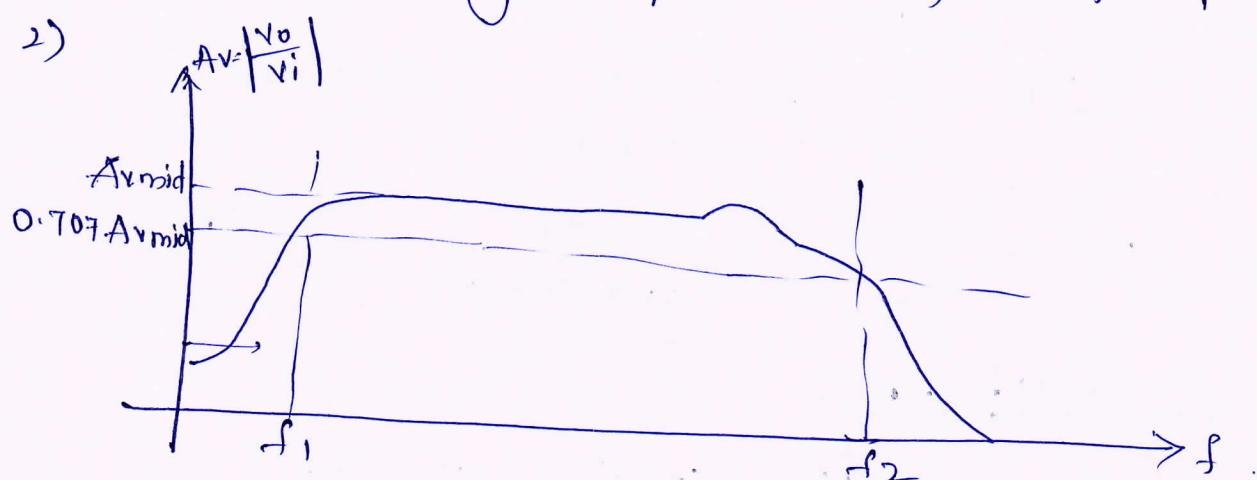
The magnetizing inductive reactance of the core is  $X_L = 2\pi f L$  & at low freq, the gain drops due to small value of  $X_L$ . At  $f=0$ , there is no change in flux in the core.
