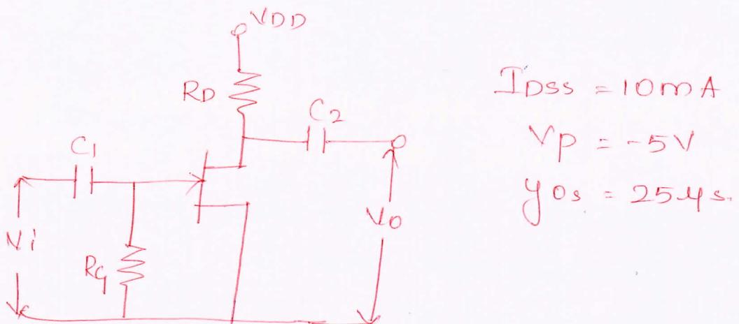
$$\rightarrow g_m = \frac{2I_{DSS}}{|V_P|} \left[ 1 - \frac{V_{GS}}{V_P} \right]$$
