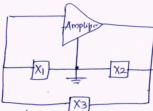
\* LC oscillators employ  $\pi$  type LC ckt to generate oscillations.
