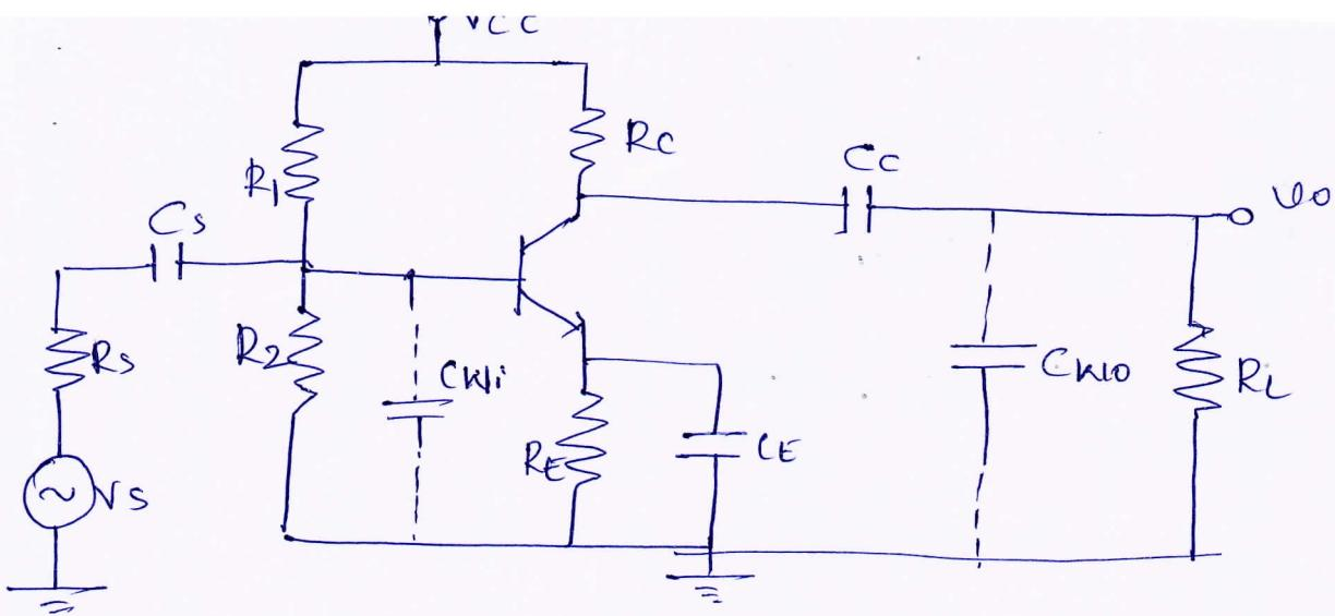
The capacitances  $C_{bc}$ ,  $C_{be}$  &  $C_{ce}$  are parasitic
