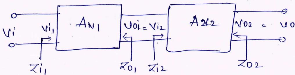
When amplification from a single stage is not sufficient, then 2 or more amplifier stages need to be connected in series. Such an arrangement is called Cascade Amplifier.
