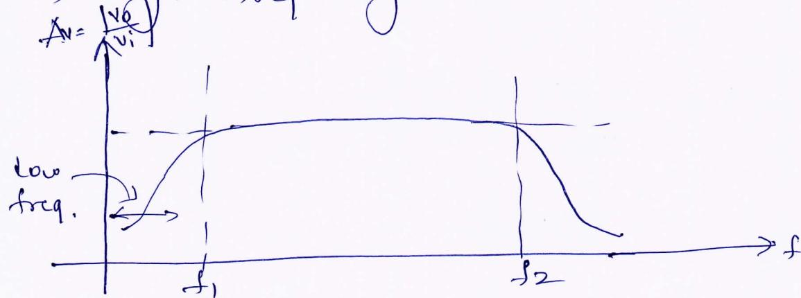
The drop in gain at low freq is due to the coupling capacitors ( $C_s$  &  $C_{s2}$ ) &  $C_E$
