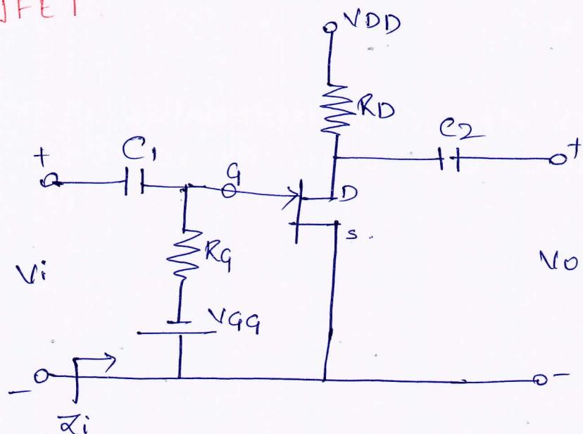
A c equivalent circuit is obtained by setting the capacitors  $C_1$  &  $C_2$  & reducing  $V_{DD}$  &  $V_{GG}$  to zero.
