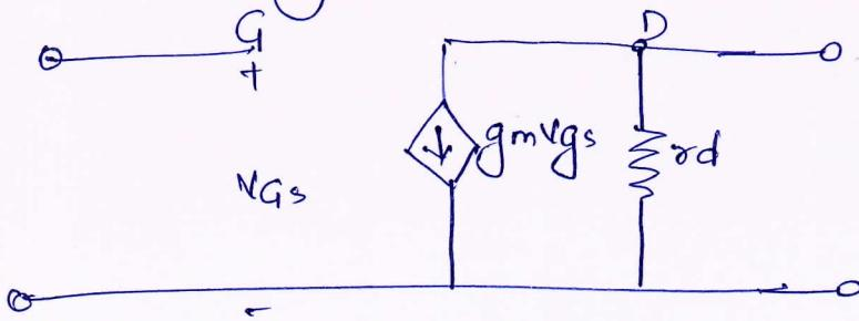
10b) Design the fixed bias FET common source amplifier shown in fig to meet the following requirements  $A_v = 12$ ,  $Z_i = 10M\Omega$ ,  $V_{DD} = 40V$
