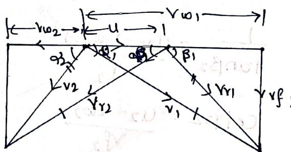
iii)  $R = 0$ .  $v_{r_1} = v_{r_2}$ .  $\beta_1 = \beta_2$
