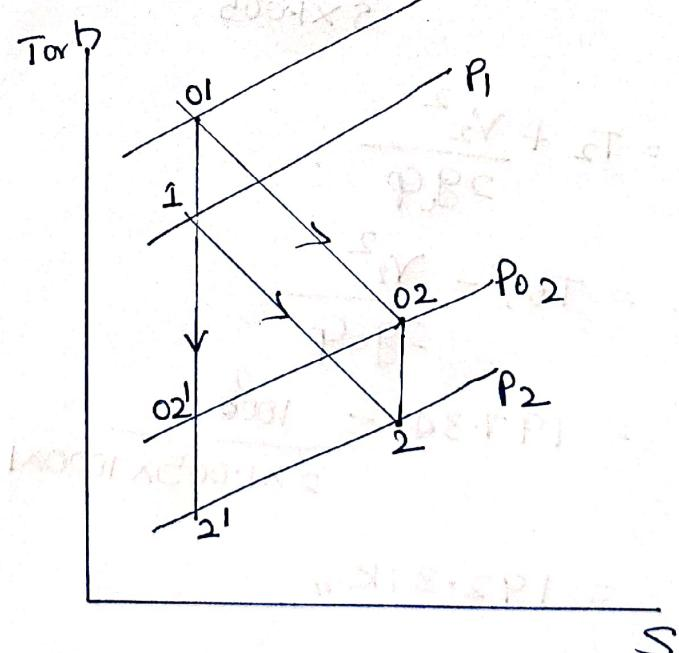
$$\frac{P_{01}}{P_{02}} = \frac{5}{1}, \quad \eta_{t-t} = 0.8, \quad m = 5 \text{ kg/s}, \quad T_{01} = 280 \text{ K},$$
