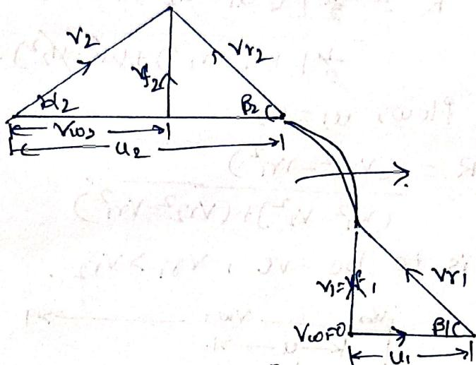
$$W.D./\text{unit mass} = (u_2 V_{w2} - u_1 V_{w1})$$
