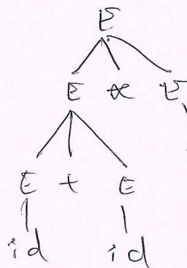
$$\text{RHS} :- \begin{array}{l} E \\ \Rightarrow E+E \Rightarrow E+E \times E \\ \Rightarrow E+E \times id \Rightarrow E id \times id \end{array}$$
