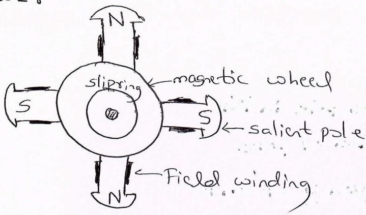
Normally it's used for 300 to 600 rpm medium speed application.
