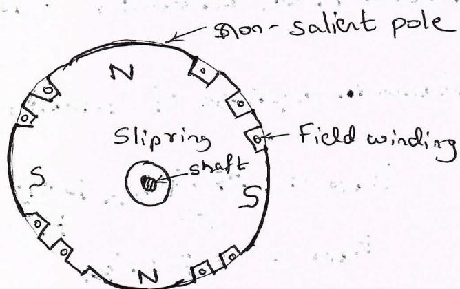
Smooth cylindrical pole rotor is used for high speed application (1500 rpm - 3000 rpm). Central polar area is isolated & flux density is maximum in that area, so it's considered as pole. It has small diameter & large axial length.
