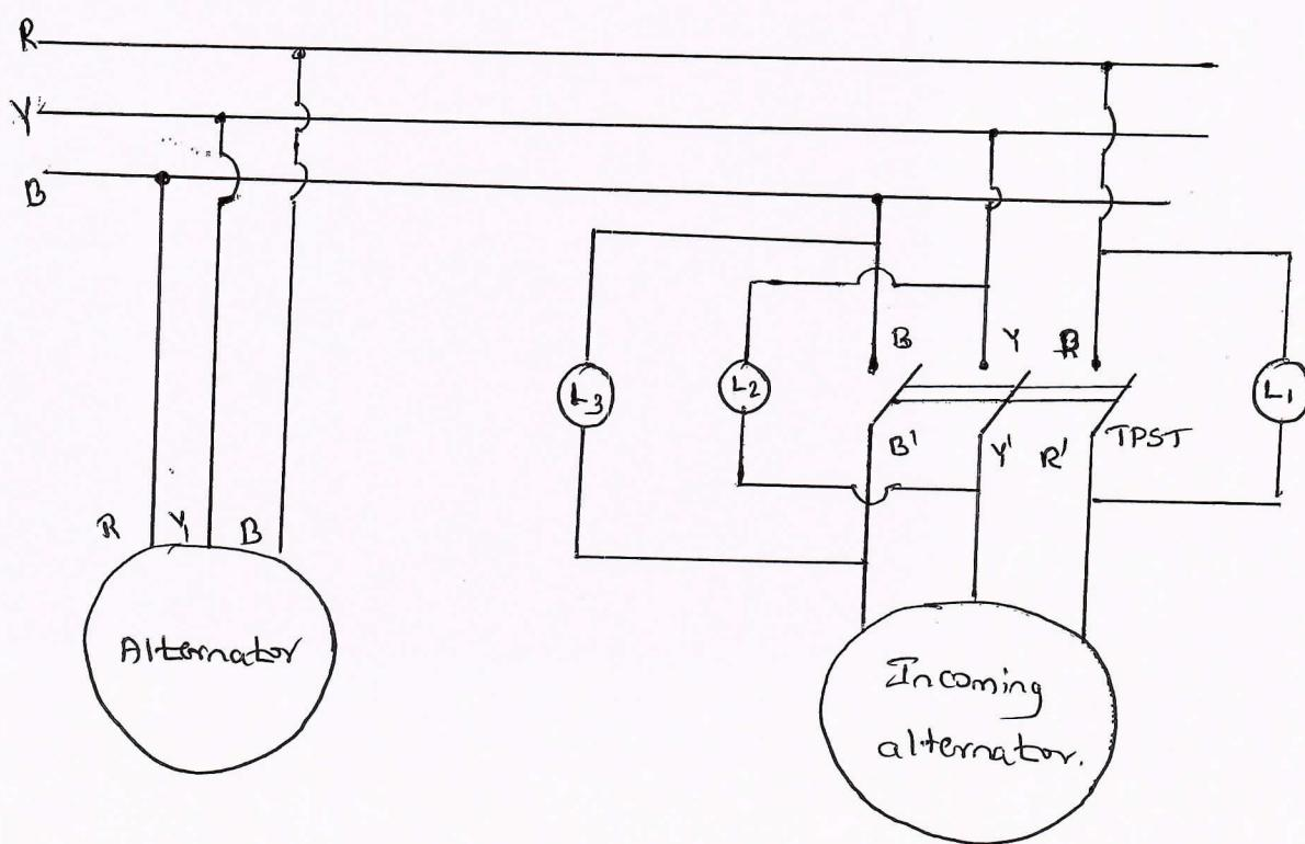
Connecting alternators in parallel to increase the capacity of the power generation is called as synchronization. Frequency, phase sequence & voltage plays vital role in synchronization.
