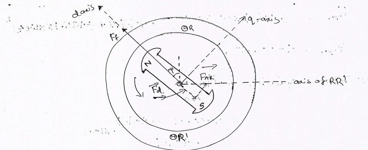
Reluctance offered in d axis is less. In q axis reluctance offered is more.  $F_f$  is the mmf wave produced by field winding. This mmf produces an excitation emf  $E_f$  which lags  $F_f$  by  $90^\circ$ . Armature produces mmf of  $F_{AR}$ . & it consists two components  $F_d$  &  $F_q$ . Armature current  $I_a$  has two components  $I_d$  &  $I_q$ .
