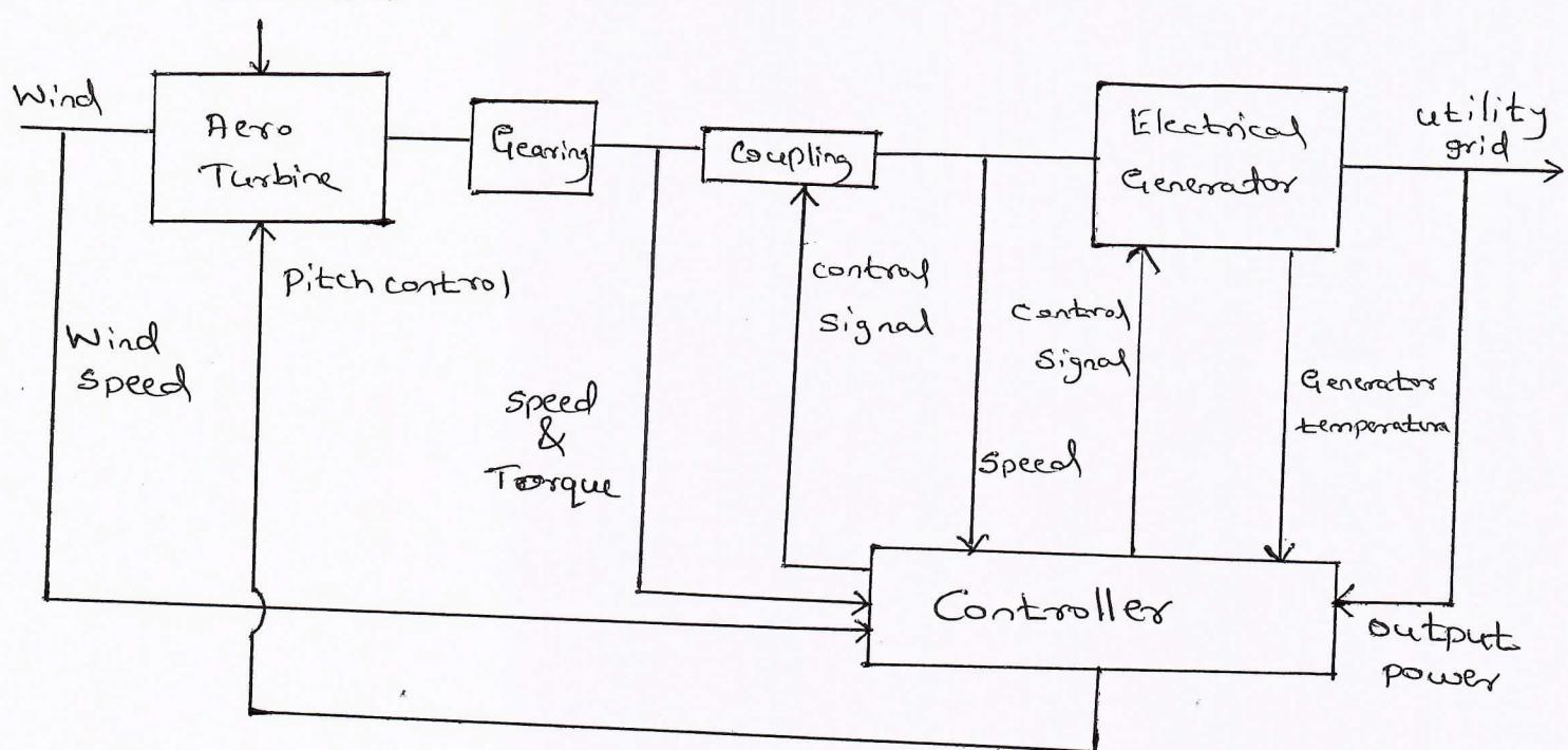
Aero Turbine → It converts energy in moving air to rotary mechanical energy. They require pitch & yaw control for proper operation.
