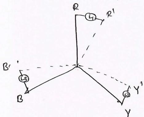
When RR', YY' & BB' get in phase with each other frequency of busbar & incoming become equal. If phase sequence is not same lamps flickers one after the other. Interchanging of two phase give solution for that. When the voltage difference between busbar & incoming generator is more, lamp brightness also more. all 3 lamp become dark, once voltage get matched. Once all 3 parameters are satisfied generators are get synchronized.
