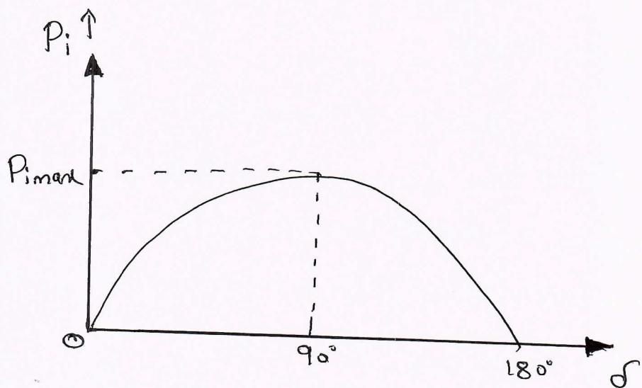
The relationship between  $P_i$  &  $\delta$  is known as power angle characteristics of the machine. The machine is normally operated at  $\delta$  much less than  $90^\circ$ .
