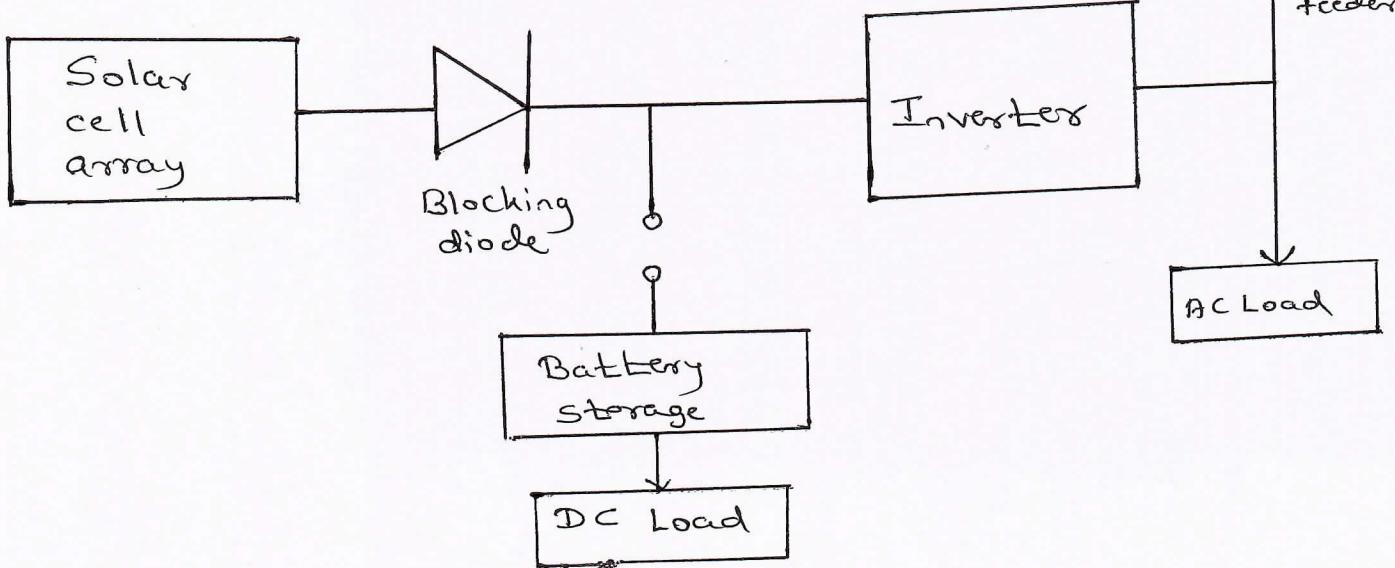
Solar Cell Array → Solar cell converts light energy into electrical energy. Number of cells are arranged in rows & columns is called as array. Set of array called as panel.
