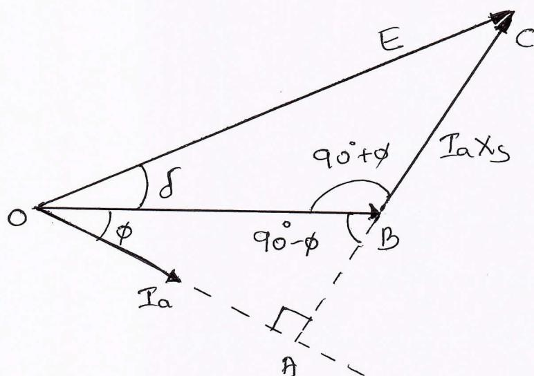
Power delivered to infinite bus  $P_i = V I_a \cos \phi$
