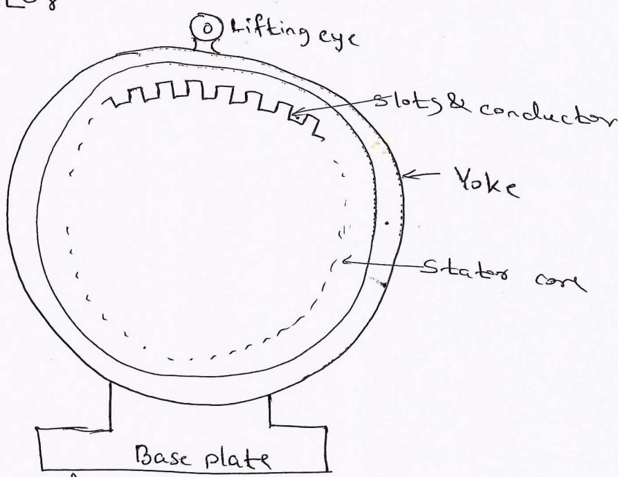
Stator is in cylindrical shape, circular laminations are jointed together to make stator core. It consists of slots to hold the conductor, which is distributed in 360°. Stator core is made up from steel or mild steel. Base-plate & lifting eye attached to stator. It acts as coreature in generator.
