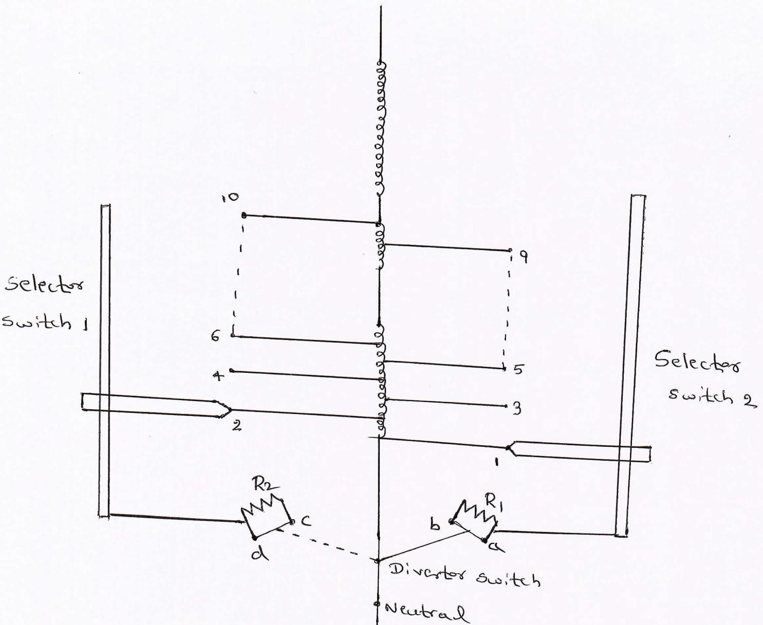
Resistors or reactors are used to ~~re~~ suppress the transients while changing the tappings.
