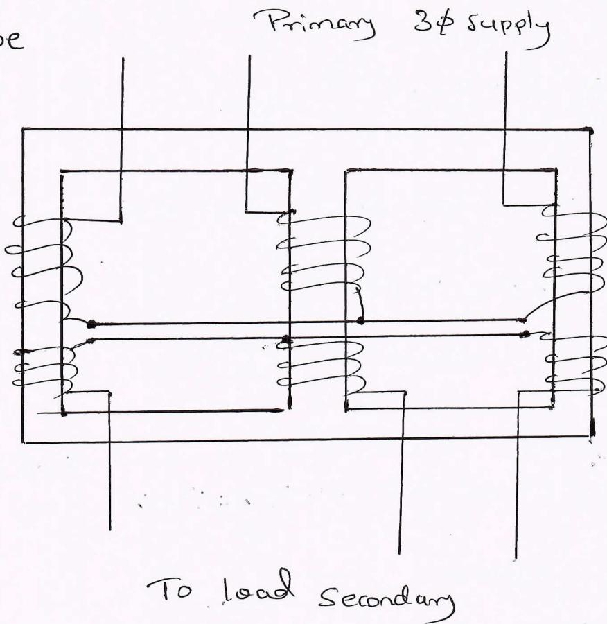
The core consists of 3 legs with magnetic circuit completed through two yokes, one at the top & the other at the bottom. Each limb has primary & secondary winding arranged concentrically. Circular cylindrical coils are used. Primary & a secondary winding of one phase are wound on one leg. Flux flows up each leg in turn & down the other two legs in general so that the magnetic circuits of different phases are in series & therefore independent.
