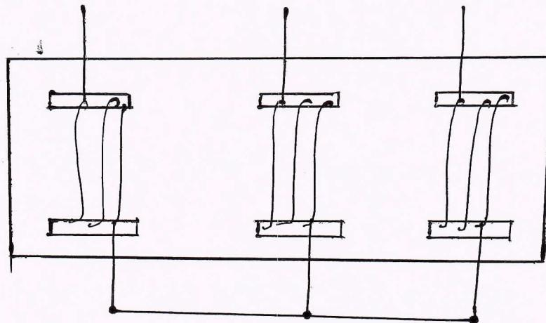
In shell type transformer the 3 $\phi$  are more independent than they are in the core type of 3 $\phi$  transformer. This is because each phase has an individual magnetic circuit which is independent of each other.
