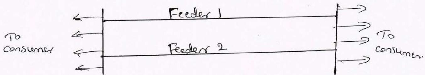
Parallel feeders reduce the elements in the radial feeder. The initial cost of this system is much more as the number ~~now~~ of feeders is doubled. Such system may be used where reliability of the supply is important.
