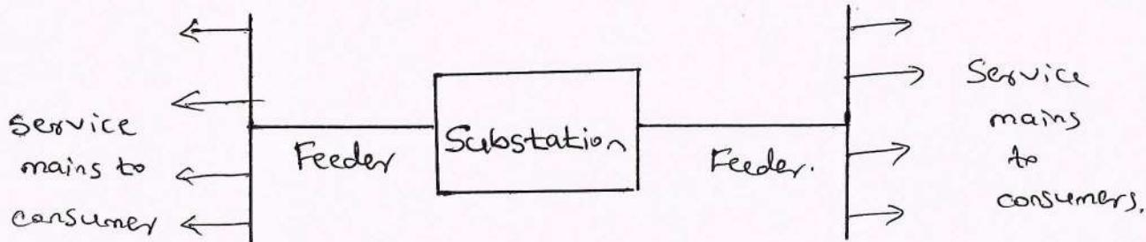
When the distributor is connected to substation on one end only with the help of feed is called as radial feeder. It's simple & less costly. End of the distributor side is heavily
