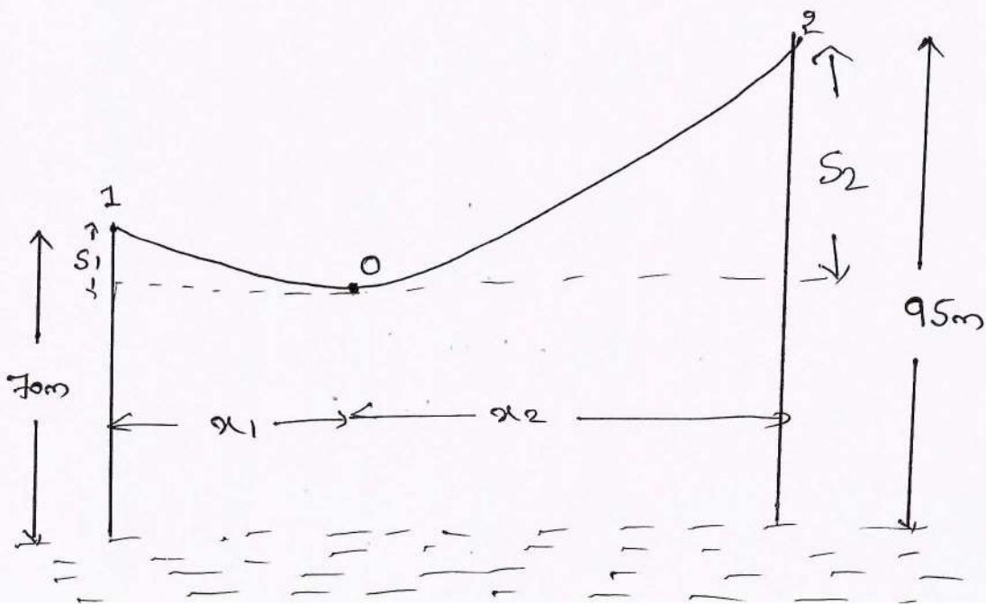
$$l = 400 \text{ m} \quad T = 1100 \text{ kg} \quad \omega = 0.8 \text{ kg/m}$$
