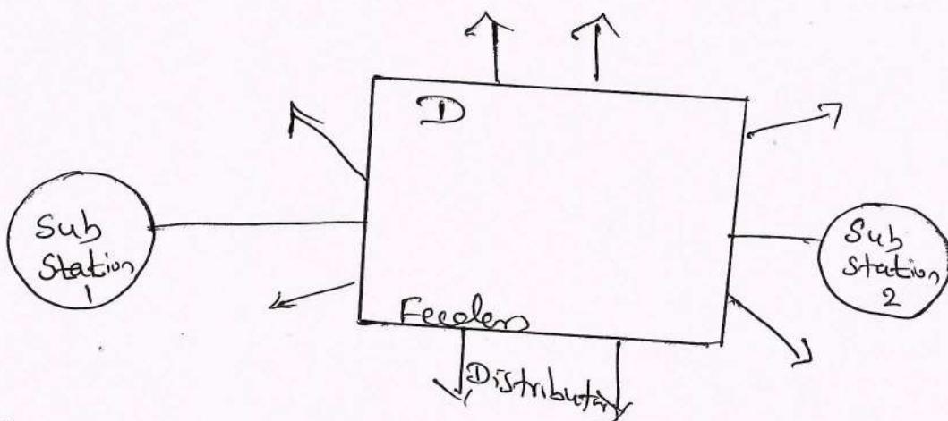
In this system substations also interconnected, like feeders. So that system can supply electricity to each consumer as per their need. Its highly reliable, but complex.
