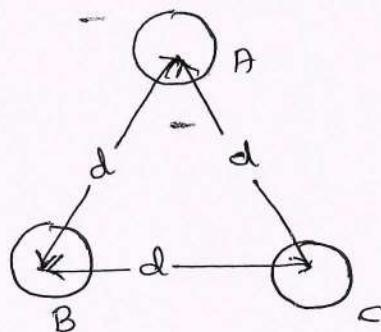
Conductor A, B & C are 'd' meters apart and  $Q_A$ ,  $Q_B$  &  $Q_C$  are charges with respective conductors.
