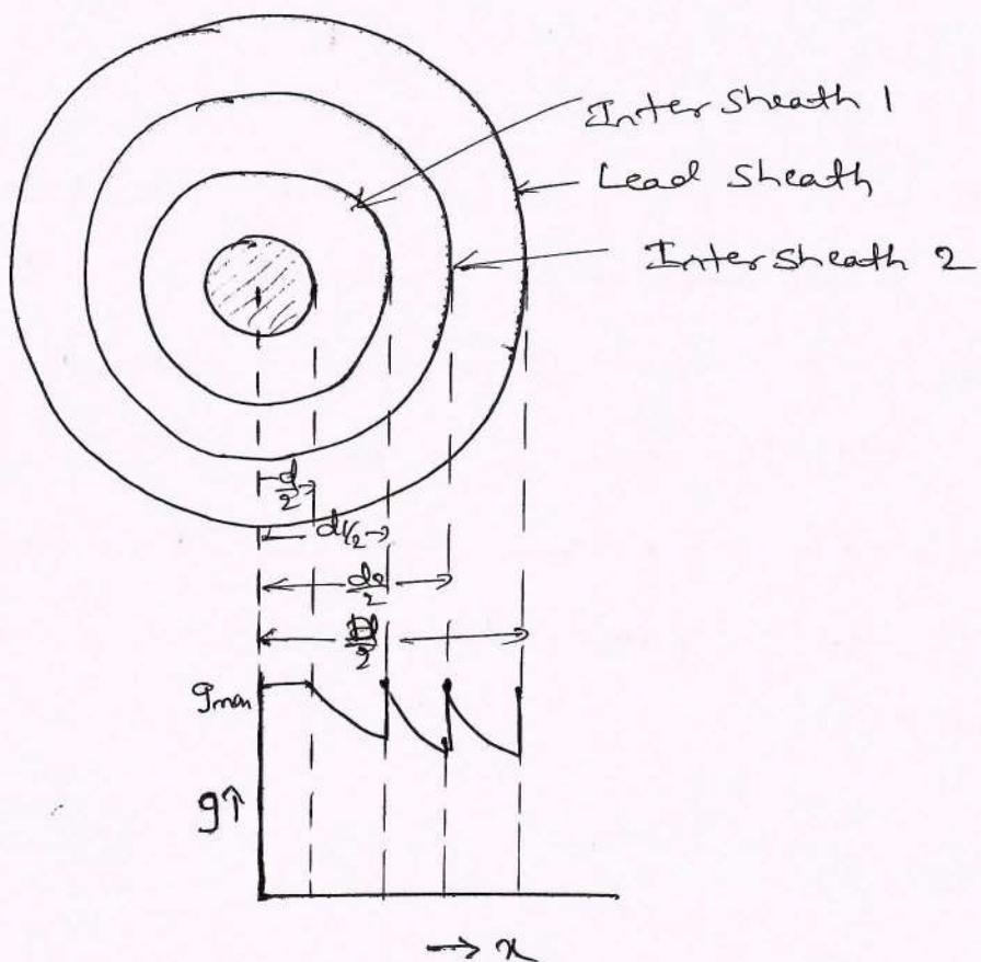
$d$  = diameter of conductors
