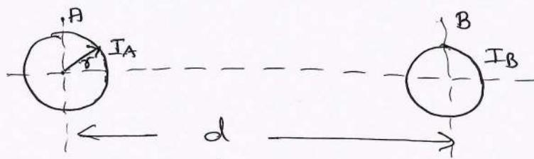
Conductor A & B placed at 'd' meter apart. 'r' is the radius of conductors.
