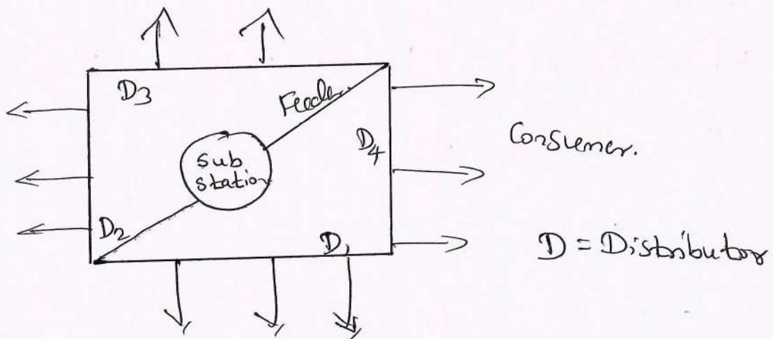
All the distributors are interconnected in loop feeders. If any one of the feeder out of service, supply will be received from another ~~fees~~ distributor. Reliability is much more higher than parallel feeders.
