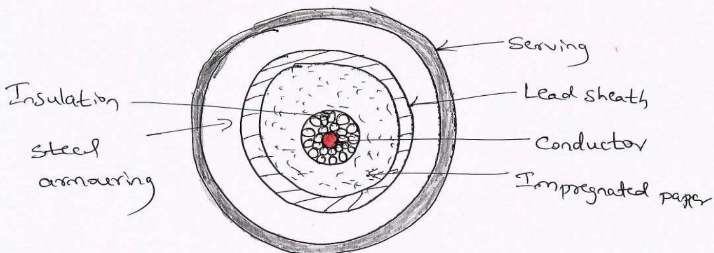
Conductor → Normally aluminum or aluminium alloy conductors are used. It consists only one core.
