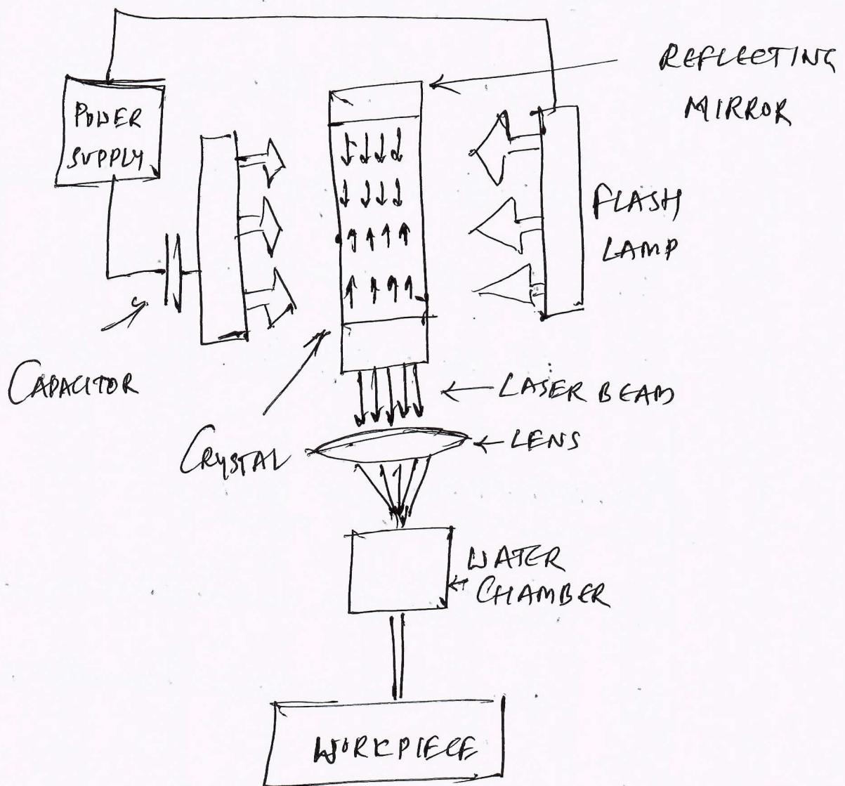
WORKING PRINCIPLE: The process consists of,
