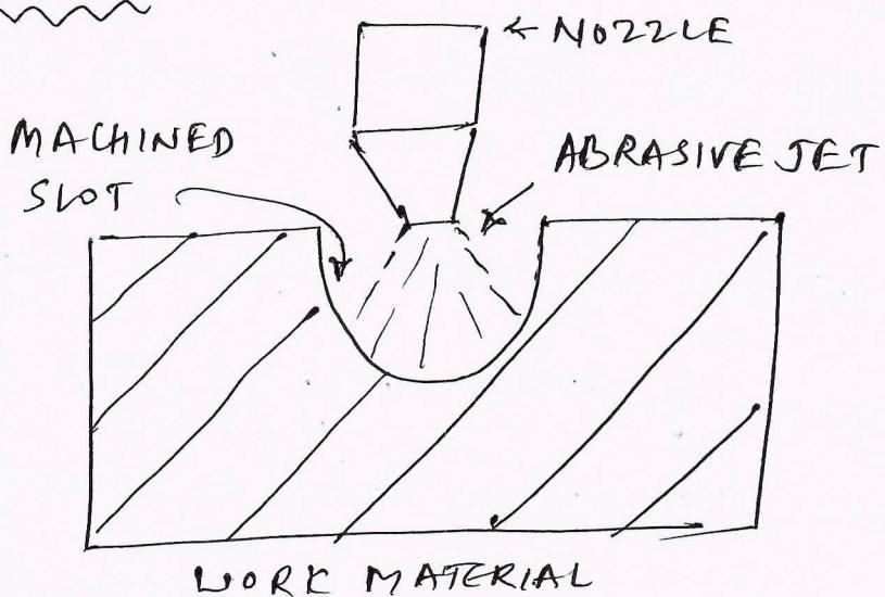
PRINCIPLE: Abrasive jet machining is the NTM process that uses a high-speed jet of abrasive particles carried by a gas to erode material from the workpiece.
