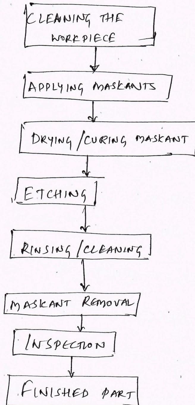
The process starts with the cleaning of the workpiece so that no foreign material on the
