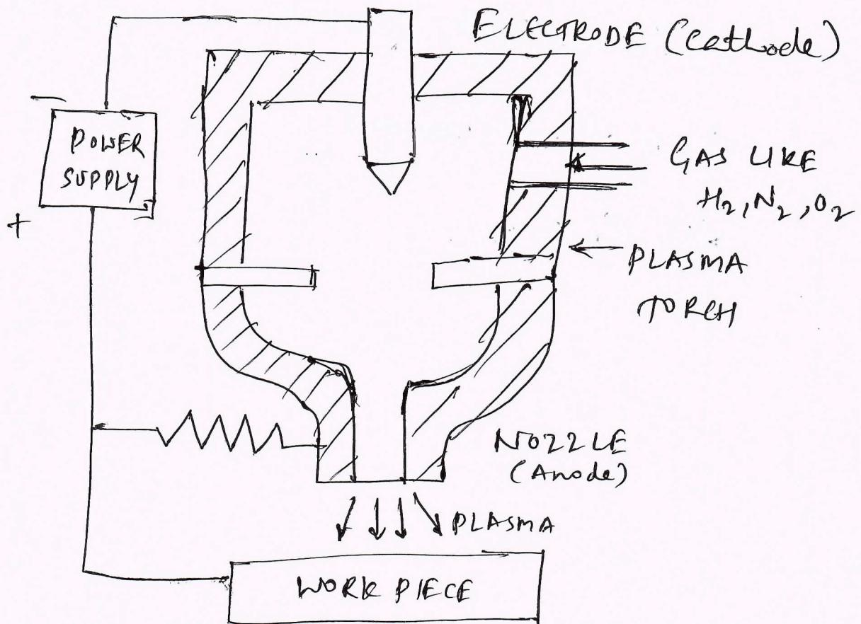
PAM is a thermal machining process that uses high temperature, high velocity jet of ionized gas (plasma) to remove material from a workpiece. The process is like,
