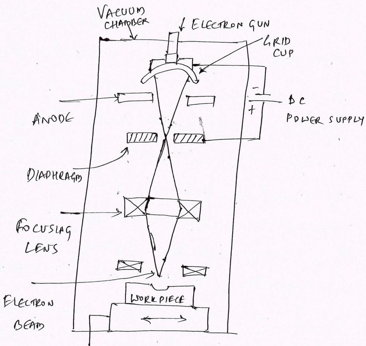
The process of EBM works as,
