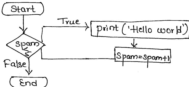
In while loop, the cond<sup>n</sup> is checked at the start of each iteration. If the cond<sup>n</sup> is true, the clause is executed & afterward, the cond<sup>n</sup> is checked again. If the cond<sup>n</sup> is false, while clause is skipped.
