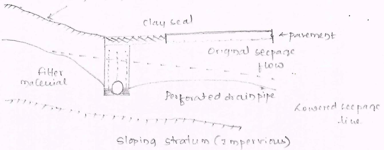
When the general ground as well as the impervious strata below are sloping, seepage flow is likely to exist. If the seepage zone is at depth less than 0.6 to 0.9 m from the subgrade level.
