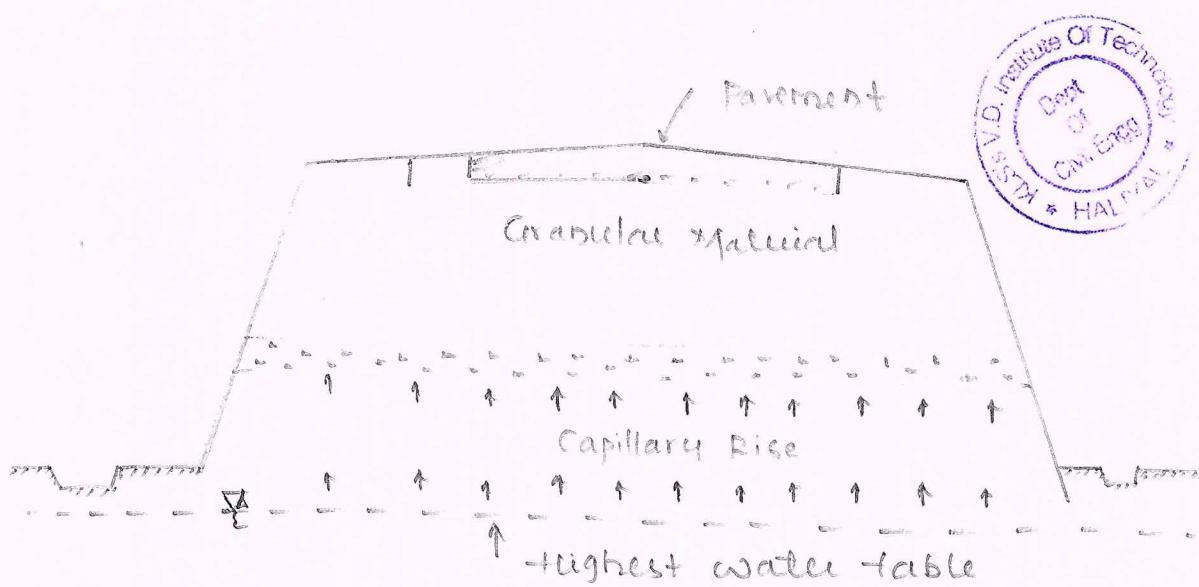
Granular Capillary cut off
