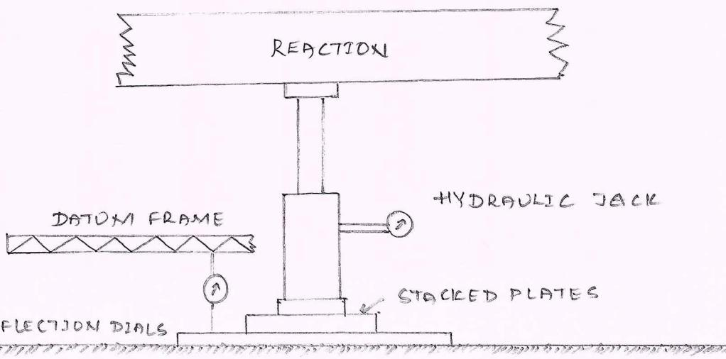
The plate bearing test is used to evaluate the support power of subgrade *in situ* for use in pavement design by using relatively large diameter plates. The plate bearing test was originally devised to find modulus of subgrade reaction in Westergaard analysis for wheel load stresses in rigid pavements.
