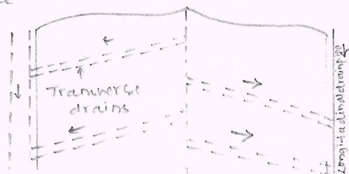
If the soil is relatively less permeable, the lowering of the ground water level may not be adequate under the centre of pavement or in between two longitudinal drainage trenches.
