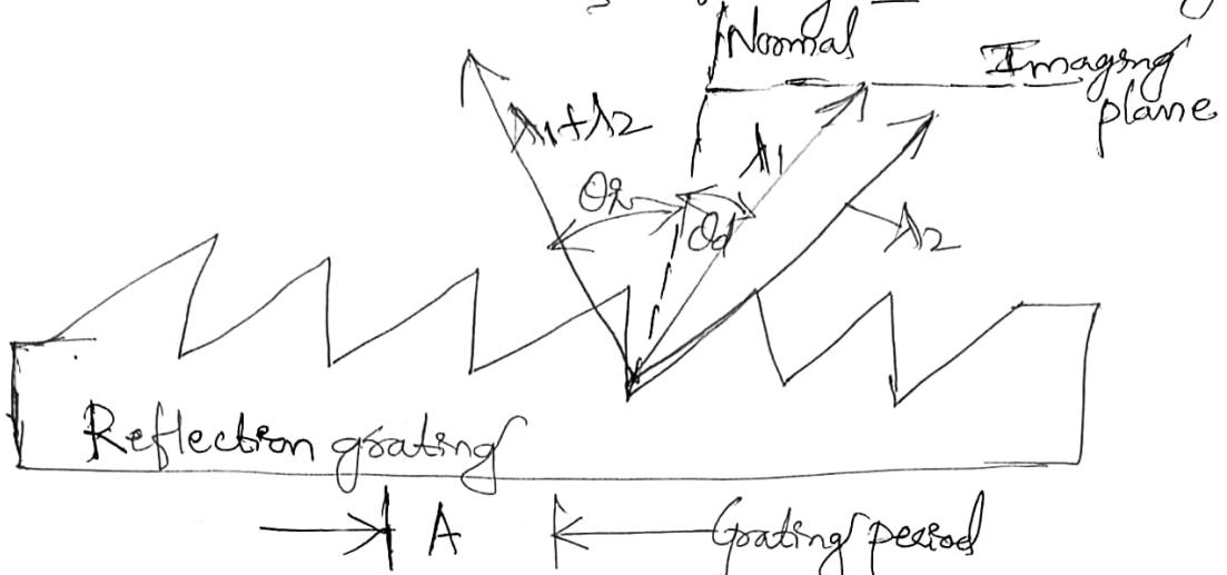
Various parameters are present for reflection grating; here  $\theta_i$  is the incident angle,  $\theta_r$  is the reflected angle,  $A$  - period of the grating. It consists of grating with equally spaced slits. Spacing between them is called pitch of the grating. Grating equation is given by  $A(\sin \theta_i - \sin \theta_r) = m\lambda$  where  $m$  - order of the grating &  $\lambda$  - wavelength.
