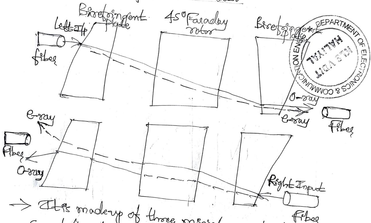
→ This is made up of three miniature optical components. The core of the device consists of  $45^\circ$  Faraday rotator that is placed between two wedge-shaped birefringent plates or walk off plates. These plates made up of  $\text{YVO}_4$  or  $\text{TiO}_2$  materials, two rays are produced ordinary ray (O-ray) & extraordinary ray (E-ray).
