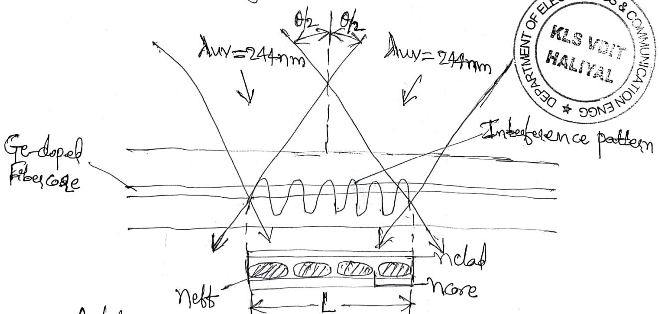
A fiber Bragg grating is a narrowband reflection filter that is fabricated through a photomasking process. One can induce the change in RI of the core by exposing it to UV radiation of  $244 \text{ nm}$ .
