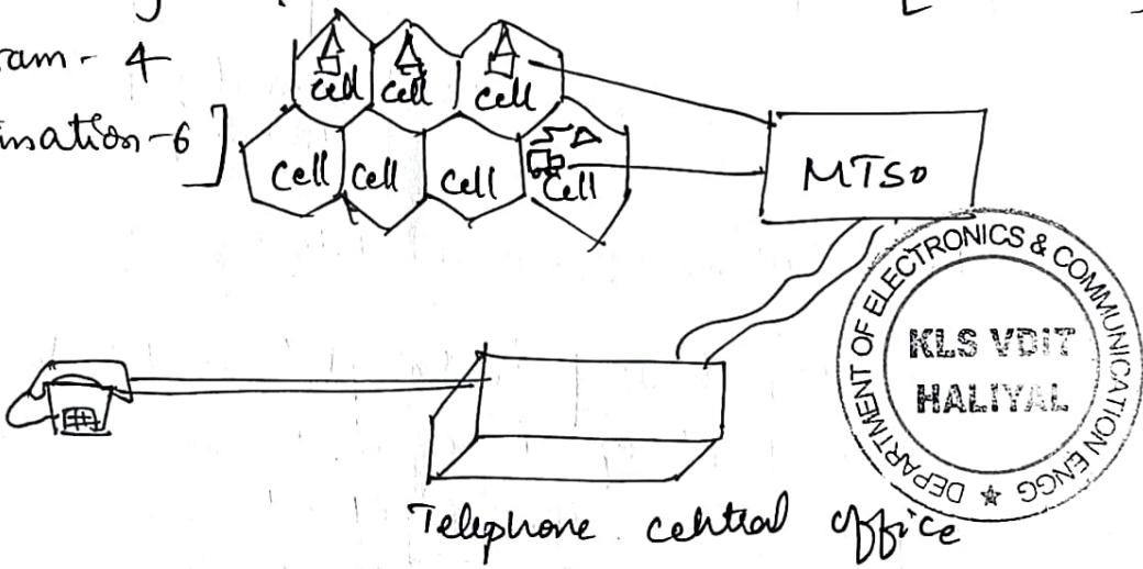
The basic cellular radio network covers a number of geographical areas (cells) connected with landline or wireless telephone communication networks deploying PSTN. Within the cell, cellular mobile subscribers can communicate with one another using the cellular network. The cellular network is defined by a set of transceivers located at the centres of each of the cells, and the locations of these radio frequency transceivers are called base stations.
