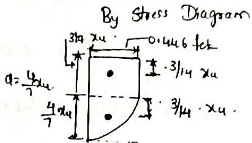
$$\text{Area of Stress block} = \boxed{\text{Base Area}} + \boxed{\text{Parabolic Area}} = \frac{3}{7} x_u \times 0.446 fck + \frac{2}{3} \times \frac{4}{7} x_u \times 0.446 fck \\ = 0.36 fck x_u$$
